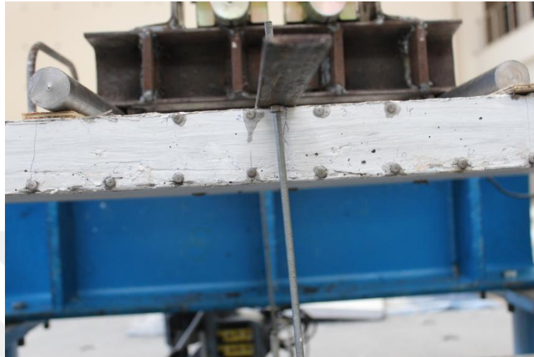
Figure 32: Beads for the four-point bending test.
