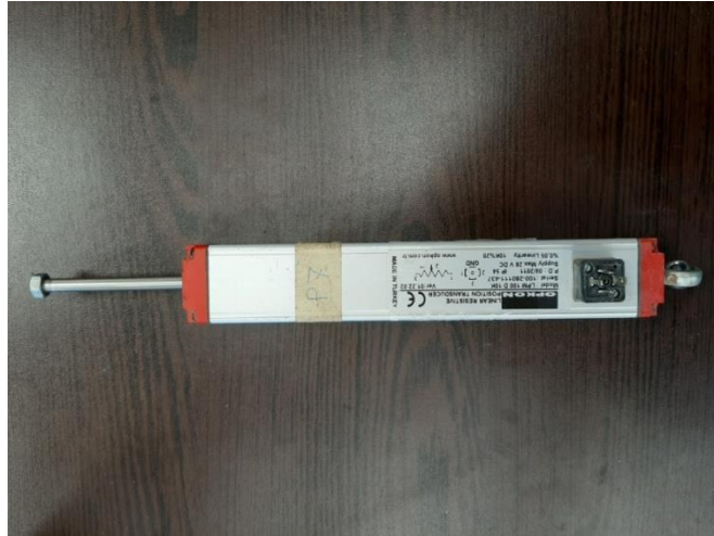
Figure 25: Linear resistive position transducer.
