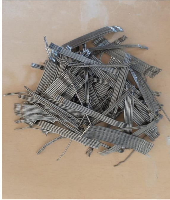
Figure 18: The used steel fiber.
