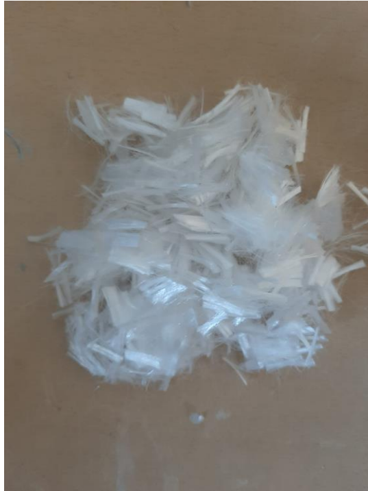
Figure 19: The used PVA fiber.
