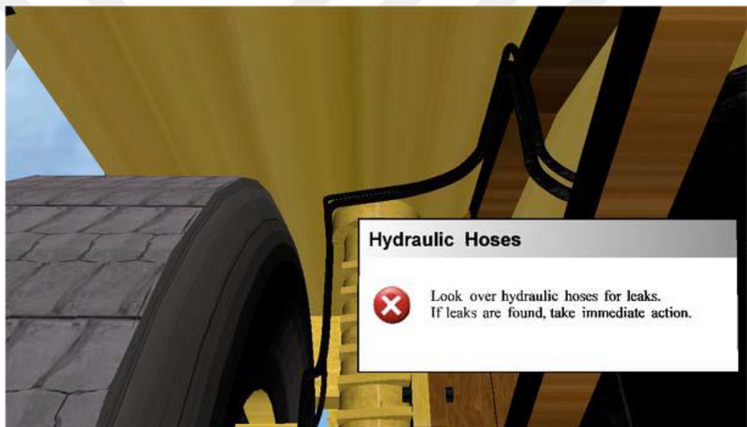
Figure 2.10. Example hydraulic hose inspection point and associated information window (McMahan et al., 2010).
