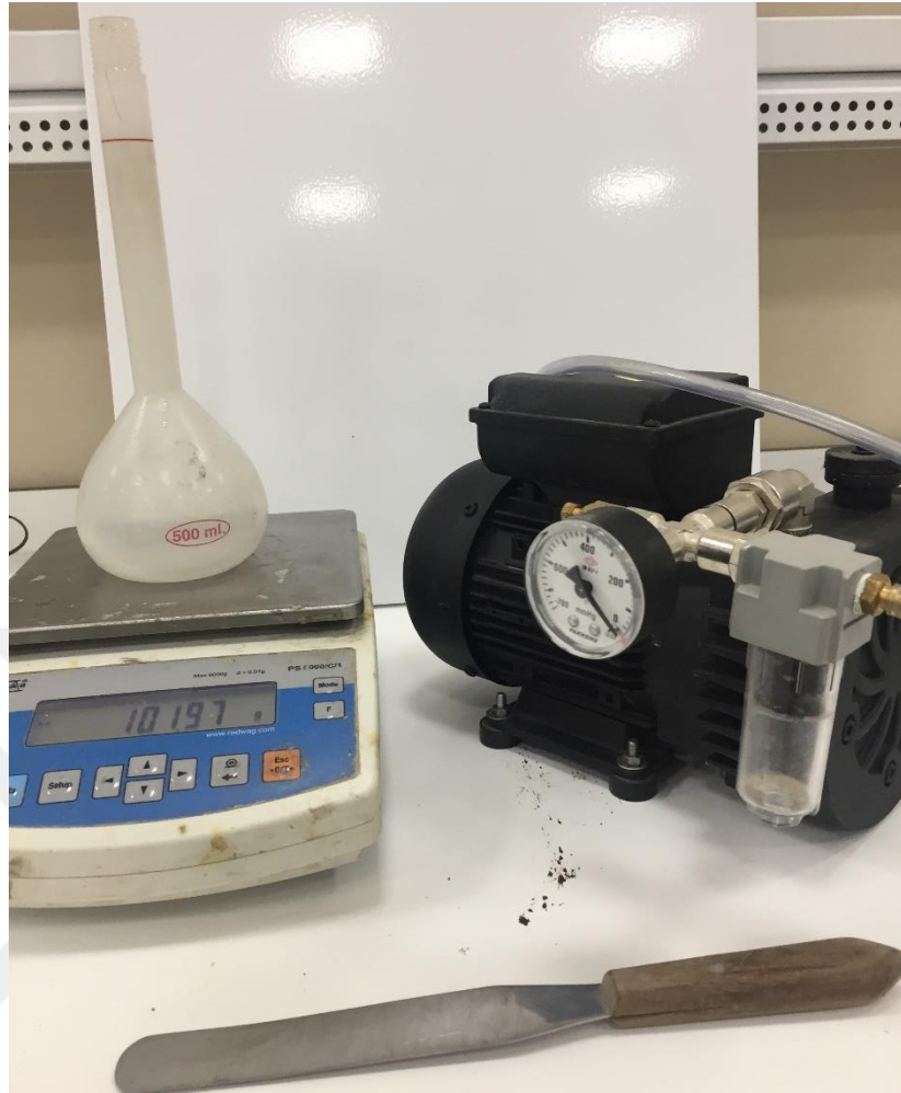
Figure 3. 8 Specific gravity test's equipment
