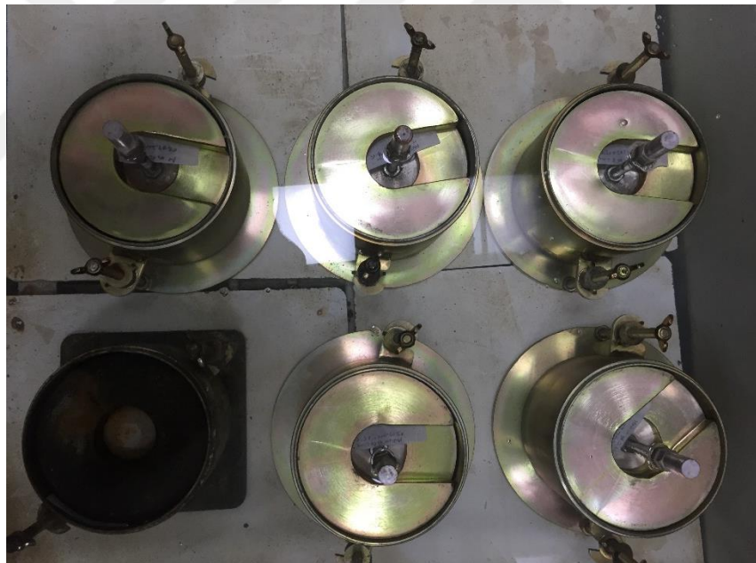
Figure 3. 16 Soaking stage of CBR test
