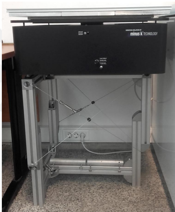
Figure 3.21. Views of an industrial-type vibration isolator (Minus K 100BM-1) and the height-adjustable support structure placed underneath.
