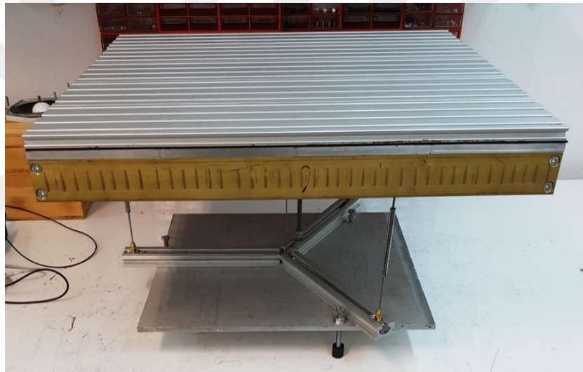
Figure 3.26. View of the large-scale isolator when brass strips are attached to the top platform to increase its mass and polar moment of inertia.
