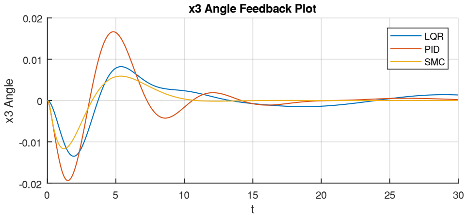
Figure 4.25. x3 angle feedback plot for x-axis with sinusoidal noise
