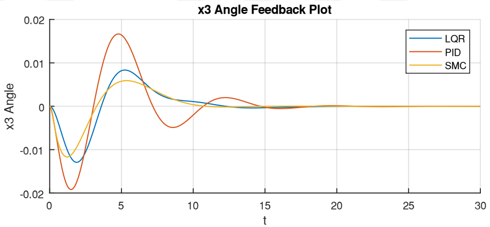
Figure 4.3. x3 angle feedback plot for x-axis with no noise
