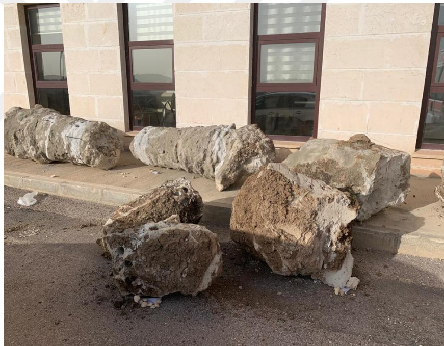
Figure 3.20 Pictures of jet grout columns
