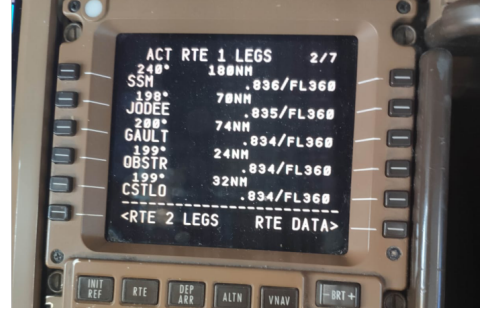
Figure 8.2 : Performance factor (left) and planned waypoints in a Flight Management Computer (right).
