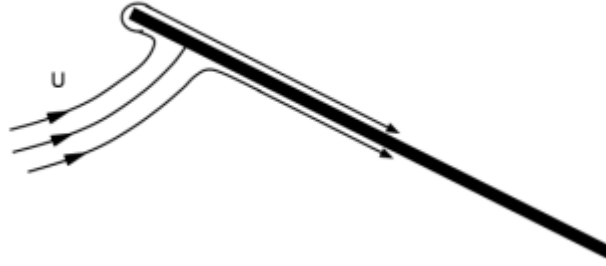
Figure 2.1: Stagnation point and the flow around the leading edge.[3]
