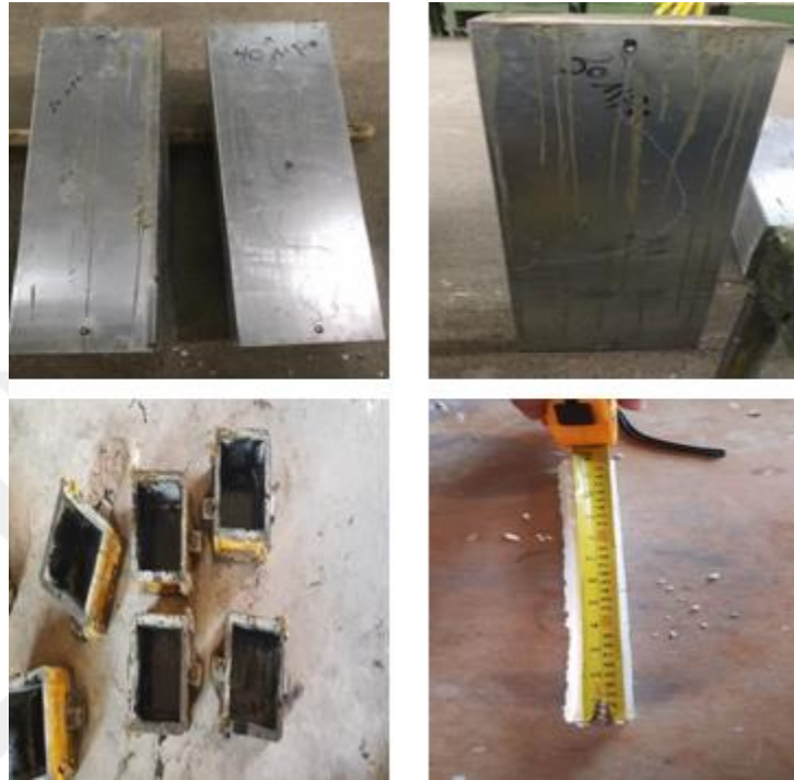
Figure 3.2. The sampling (20 Mpa, 30 Mpa, 40 Mpa) and the dimensions damages.
