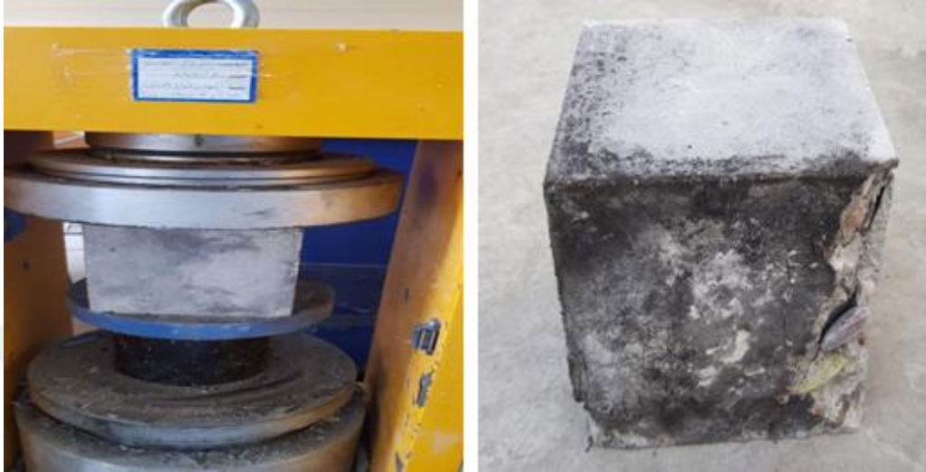
Figure 3.5. Test of Compressive Strength and Cubes Failed.
