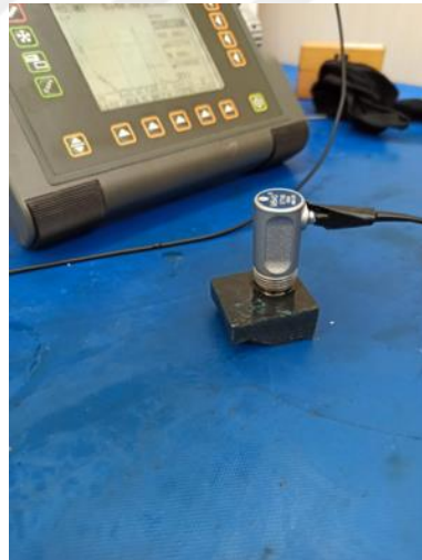
Figure 2.21 Measurement of the longitudinal wave of PMMA/GNPs 1% Nanocomposite with MB4S probe.
