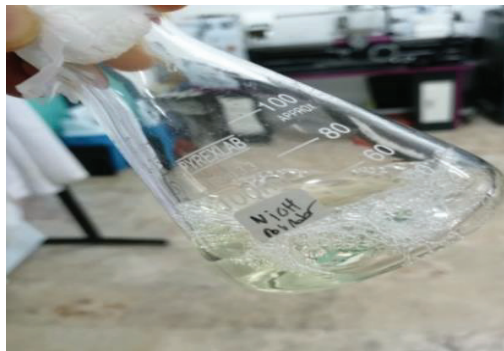
Figure 2.2. Example of binder (glue) for nickel hydroxide
