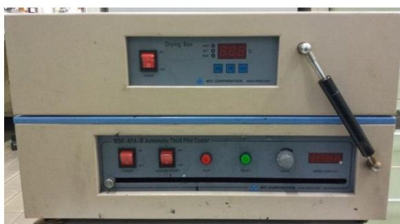
Figure 3. 6 Heater for drying electrode
