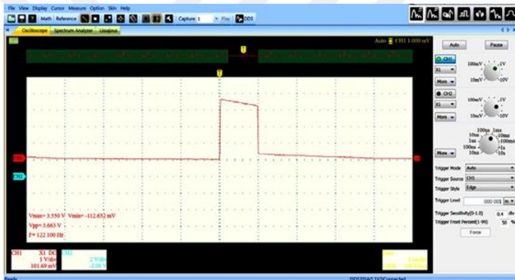
Figure 7.15. Real oscilloscope presenting for the received laser pulse at the output of the 50 Hz Notch Filter.
