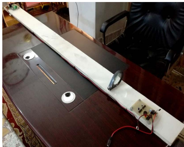
Figure 6.7. The practical prototype of the 50 meter laser FSO communication link.
