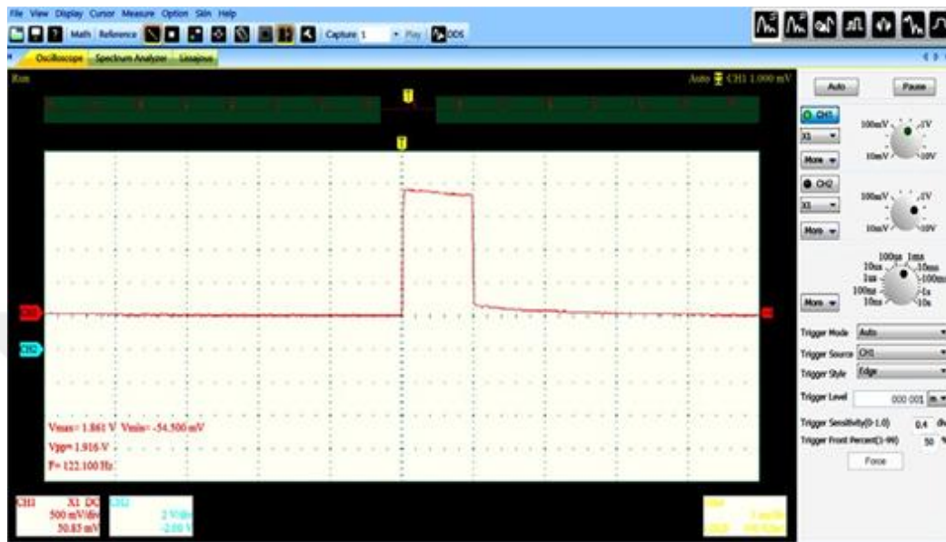
Figure 7.14. Real oscilloscope presenting for the received laser pulse at the output of the Low Noise Amplifier.
