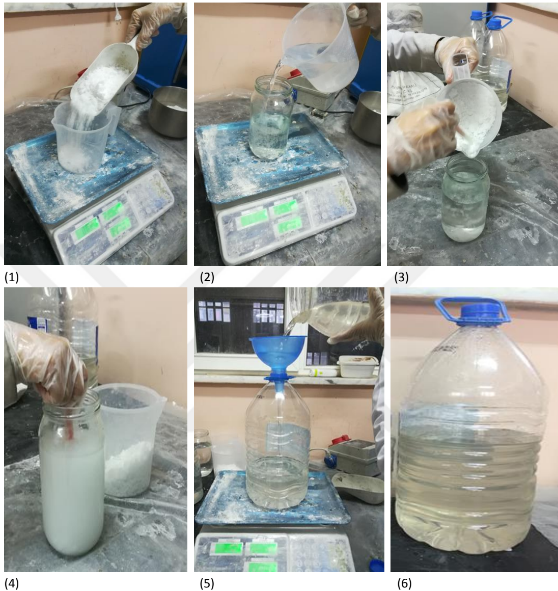
Figure 3.8 Preparation of alkaline solution
