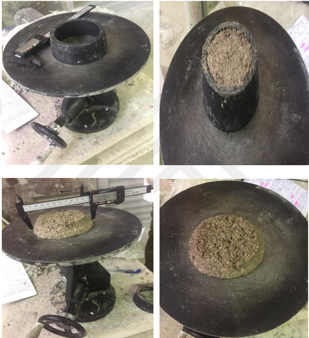
Figure 3.12 Flow table test of lightweight geopolymer mortar
