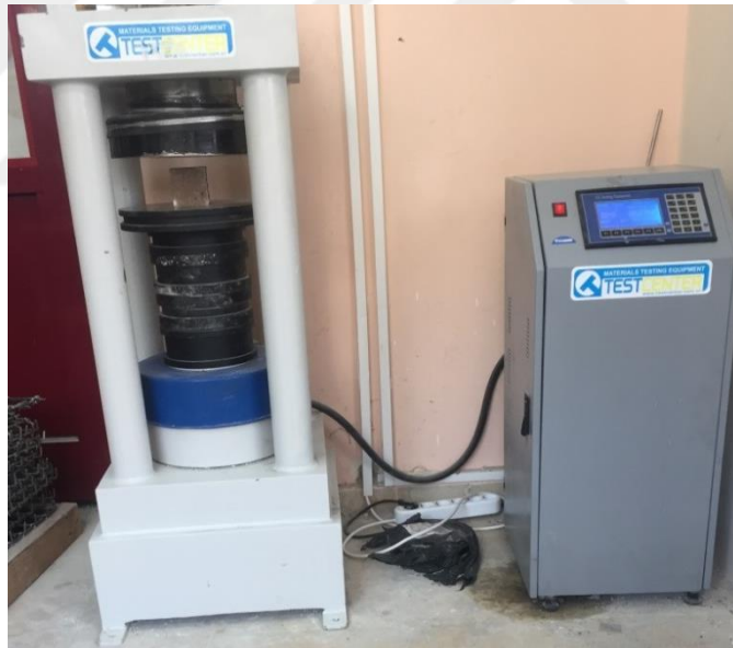
Figure 3.14 Compression test of a cube specimen
