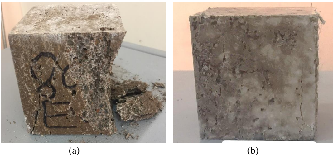
Figure 4.5 Failure modes of cube samples after compression test. (a) 80%EC ;(b) 80%EC-1%PVA
