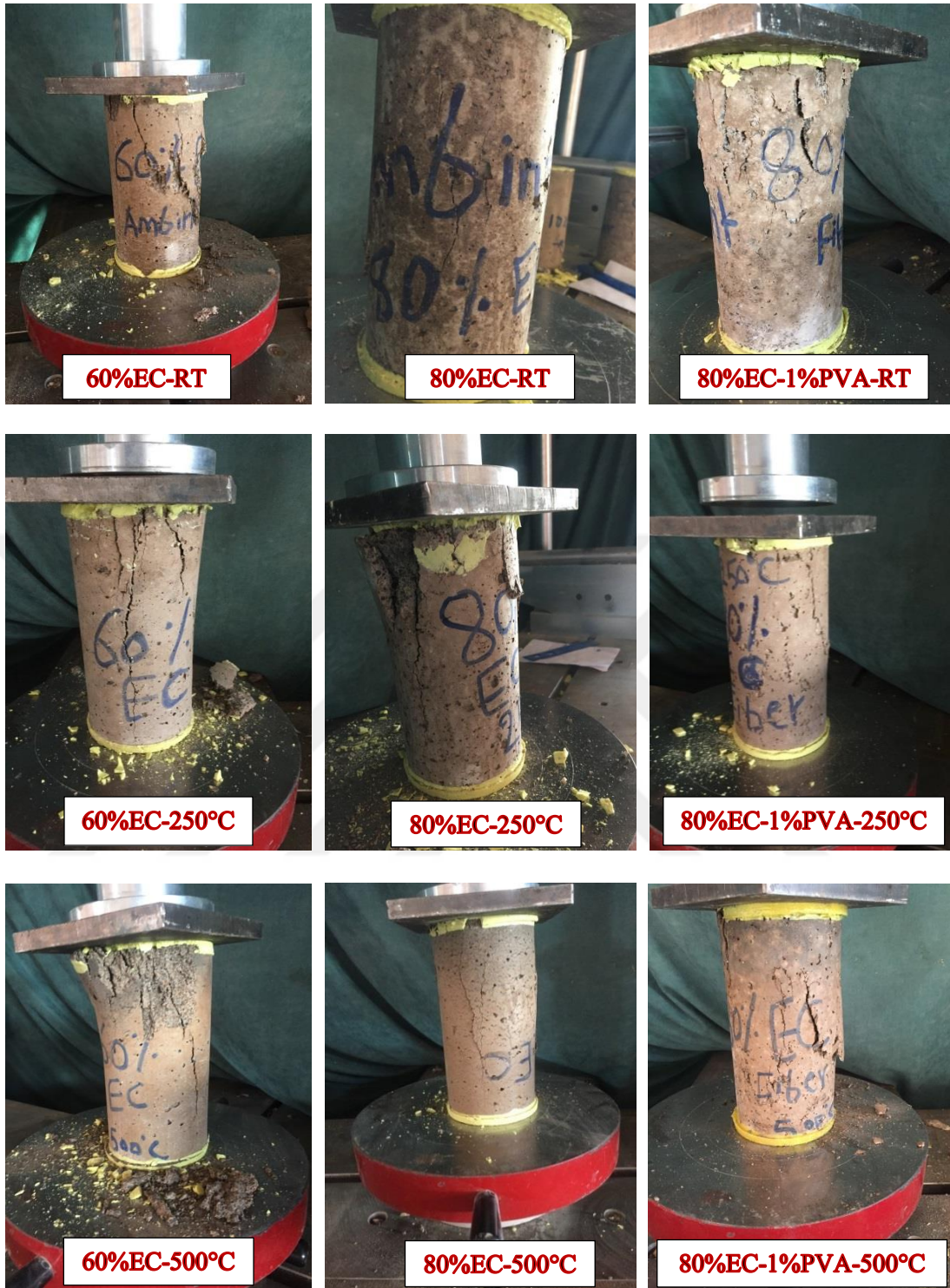
Figure 4.8 Failure patterns of cylinder samples under different temperatures (RT: Room temperature)
