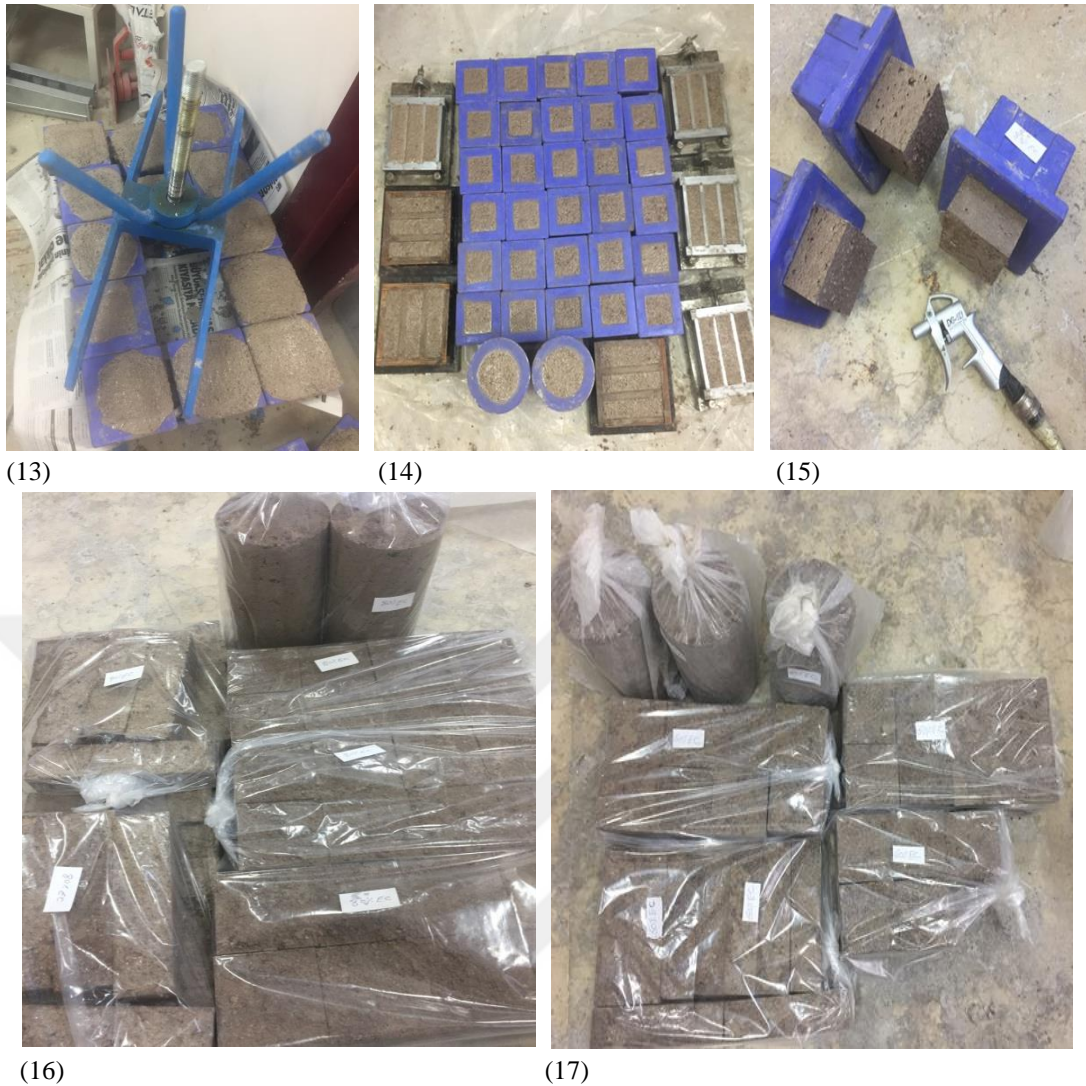
Figure 3.9 Mixing, casting and curing of samples without fibers
