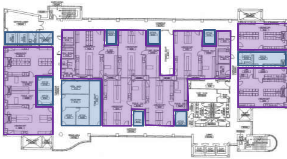
Figure 4.2: The floor-layout for the 3rd and 4th floors of the Central Hospital Istanbul where the entire floor serves as laboratory spaces.
