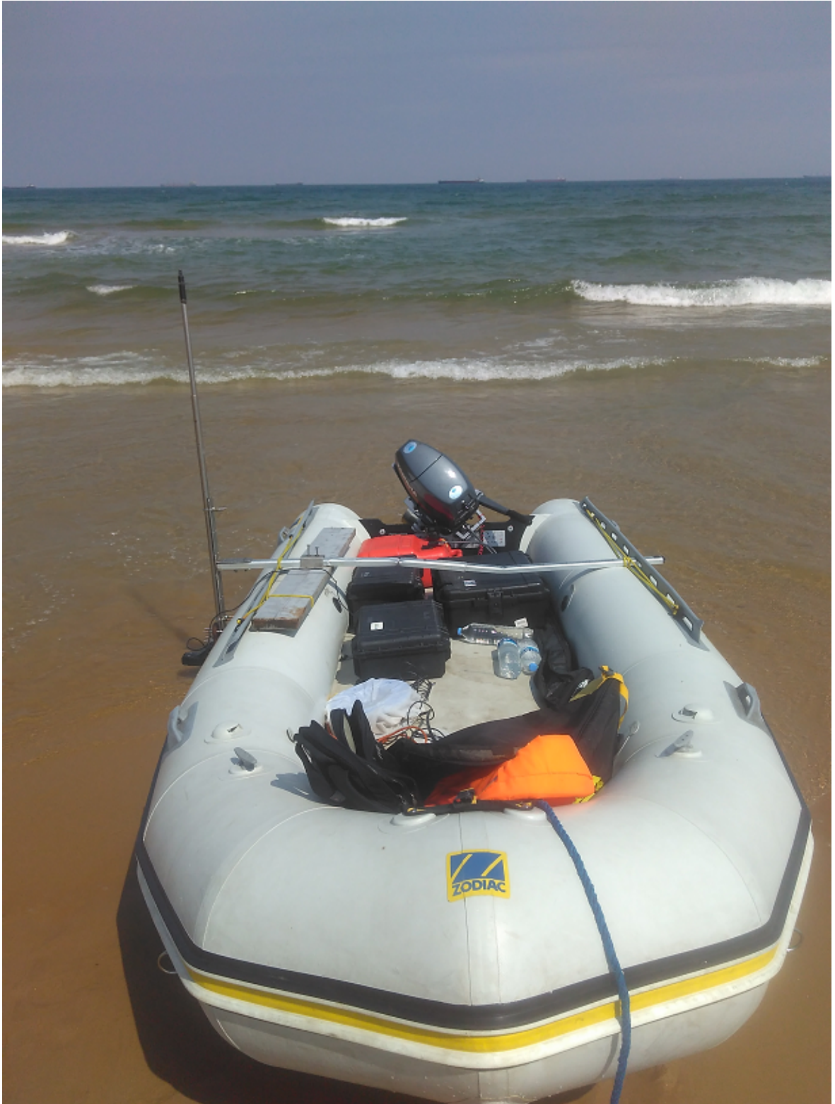
Figure 2.2. Survey boat with pole for GNSS receiver and echo sounder, Aug 22, 2016 (preparation survey).
