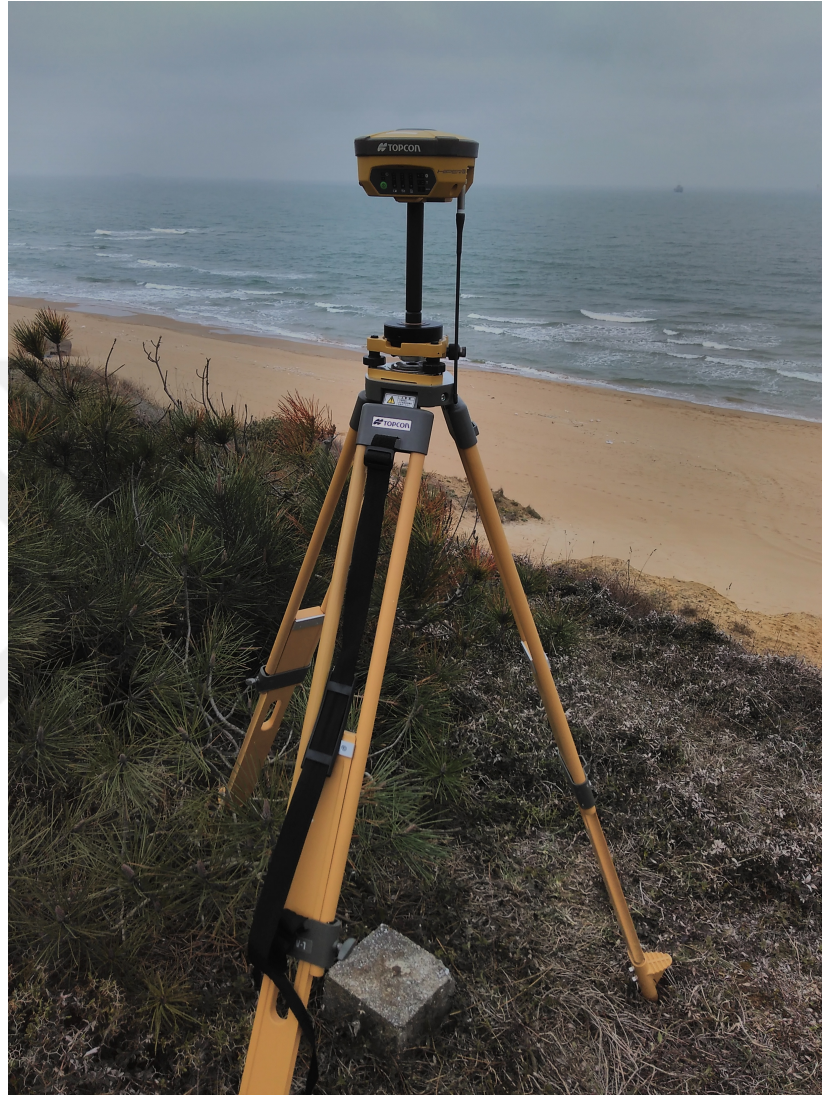
Figure 2.1. Base GNSS receiver, March 24, 2017 (preparation survey).
