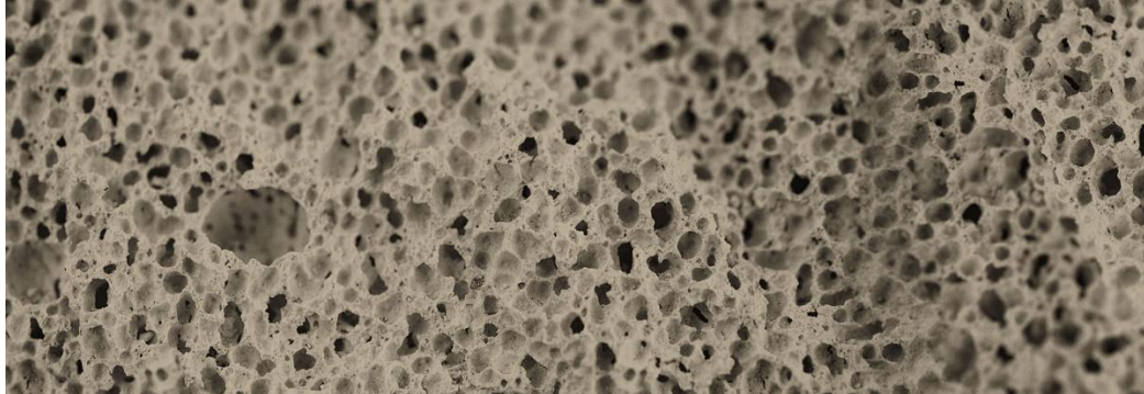
Figure 1.4: Porous Structure of AAC (Imber, n.d.)
