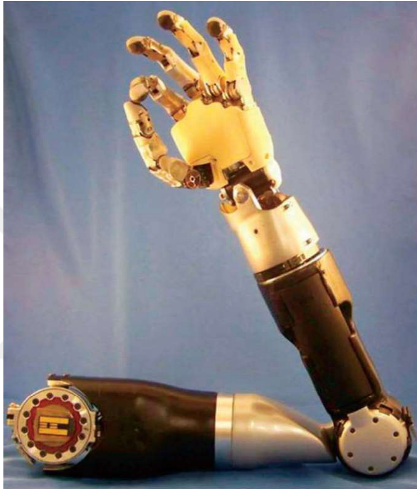
Figure 2.5: State of the art Modular Prosthetic Limb by John Hopkins Applied Physics Laboratory, USA [Johannes et al., 2011]
