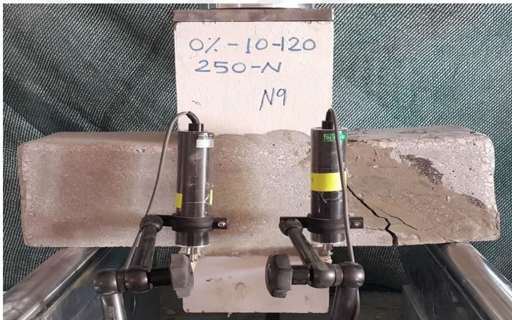
Figure 4.2 Specimen (C1-0.0-250) failure before repairing
