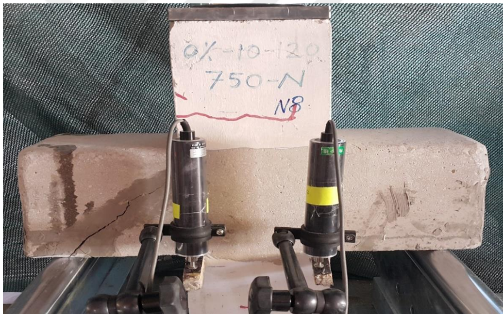
Figure 4.8 Specimen (C3-0.0-750) failure before repairing
