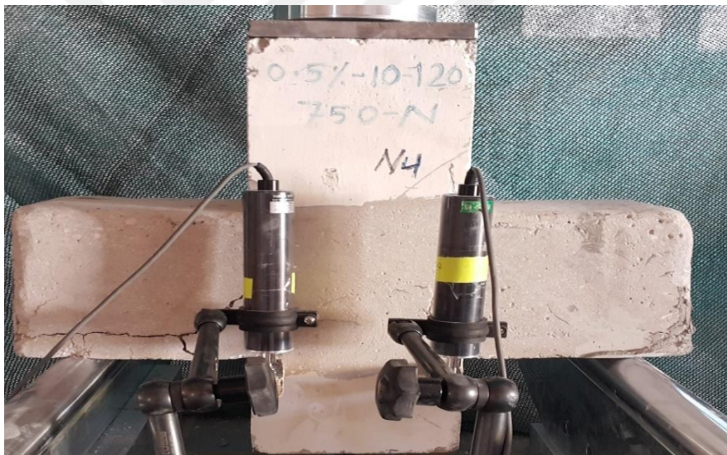
Figure 4.17 Specimen (C6-0.5-750) failure before repairing
