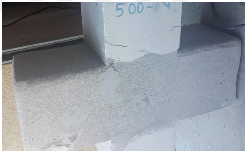
Figure 3.11 Surface preparation before gluing the basalt fiber
