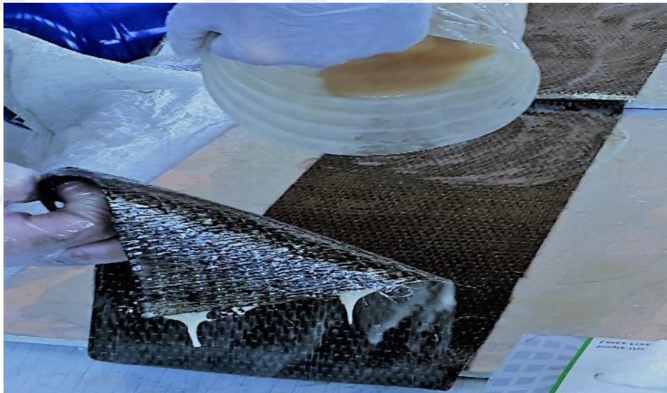
Figure 3.13 Saturated basalt fiber with low epoxy
