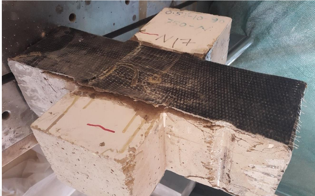
Figure 4.45 Specimen (C15-0.5-750 ) de-bonding failure after strengthening
