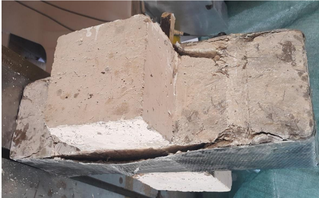
Figure 4.36 Specimen (C12-0.0-750 ) de-bonding failure after strengthening C13-0.5-250:
