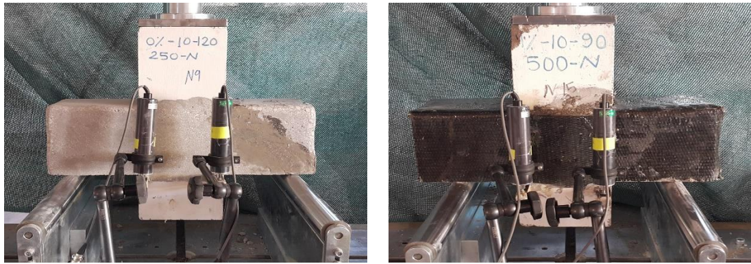
Figure 3.17 Injected and covered corbels with two LVDTs on the testing machine
