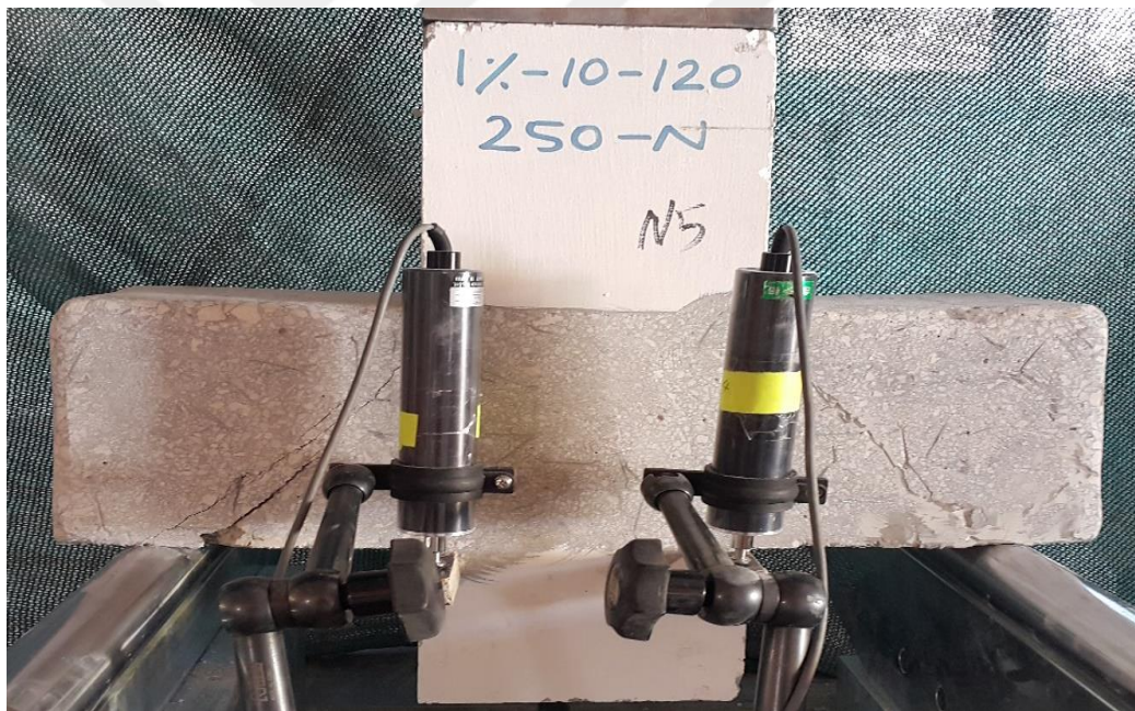
Figure 4.20 Specimen (C7-1.0-250) failure before repairing
