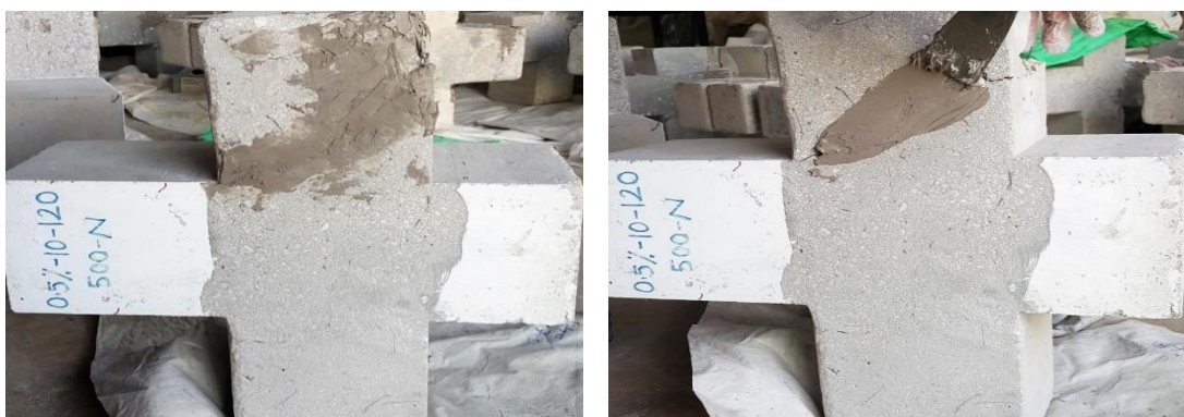
Figure 3.8 Filling the side cracks with high viscosity epoxy
