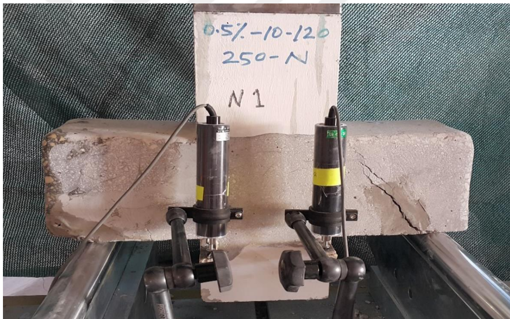
Figure 4.12 Specimen (C4-0.5-250 ) after repairing
