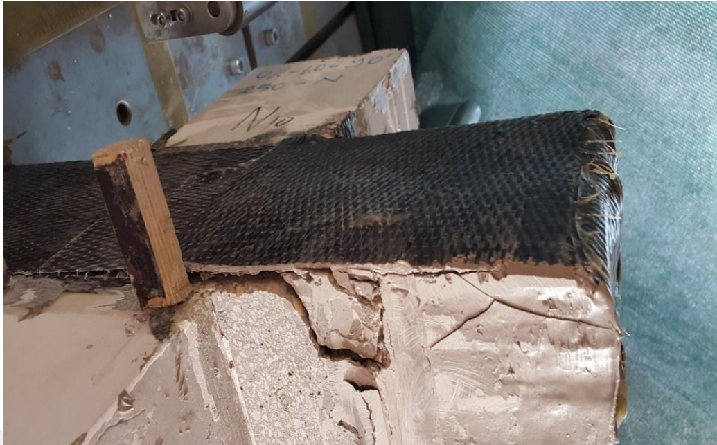
Figure 4.30 Specimen (C10-0.0-250 ) de-bonding failure after strengthening
