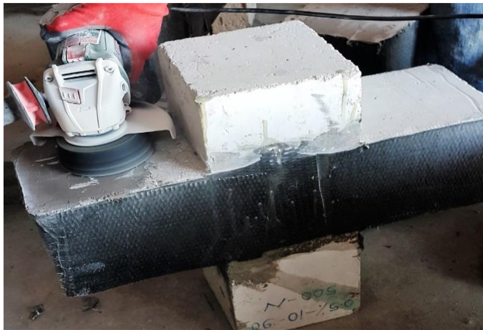
Figure 3.15 Grinding after covering of basalt fiber
