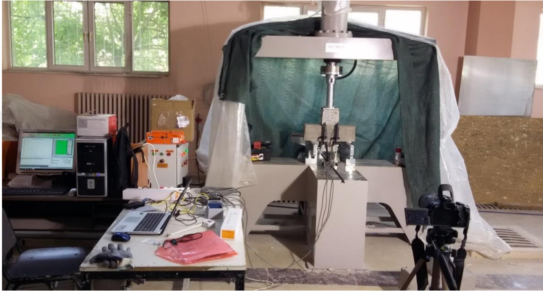
Figure 3.16 Corbel Specimen Setup.
