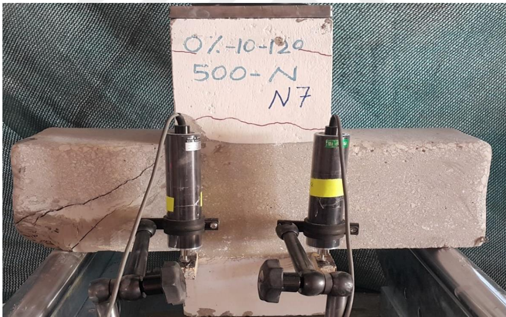
Figure 4.6 Specimen (C2-0.0-500 ) failure after repairing
