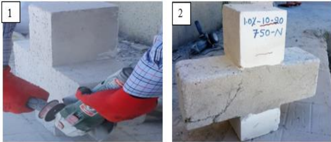
Figure 3.5 Surface grinding process
