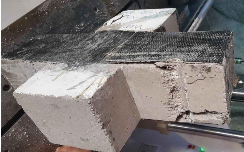
Figure 4.42 Specimen (C14-0.5-500 ) de-bonding failure after strengthening C15-0.5-750:
