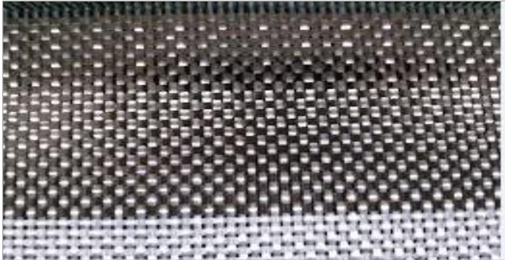
Figure 2.4 Typical Basalt Fibers Reinforced Polymer (BFRP)
