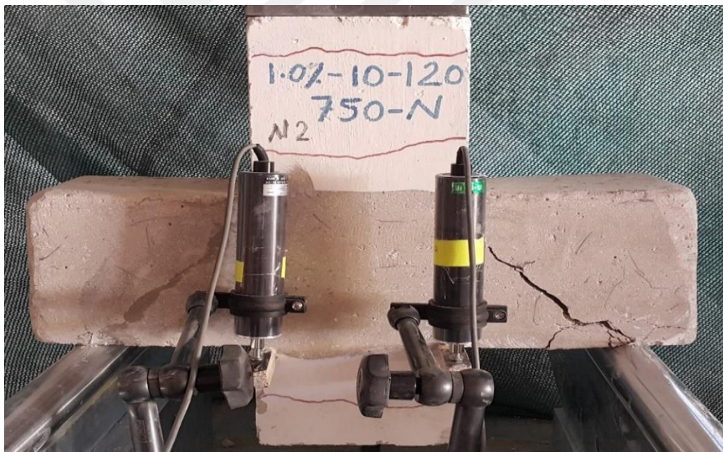
Figure 4.27 Specimen (C9-1.0-750 ) failure after repairing
