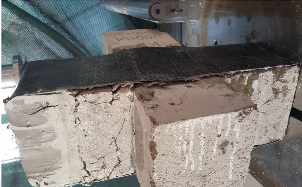
Figure 4.51 Specimen (C17-1.0-500 ) de-bonding failure after strengthening
