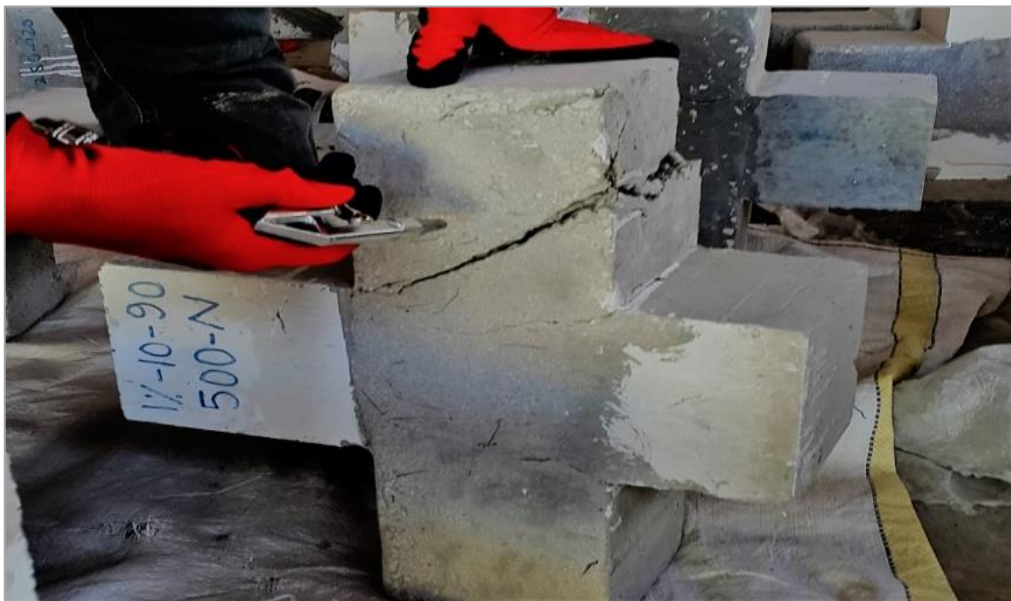
Figure 3.6 Using air compressor for removing loose particles
