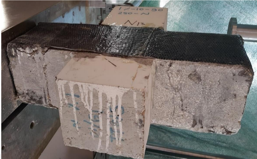
Figure 4.48 Specimen (C16-1.0-250 ) de-bonding failure after strengthening C17-1.0-500:
