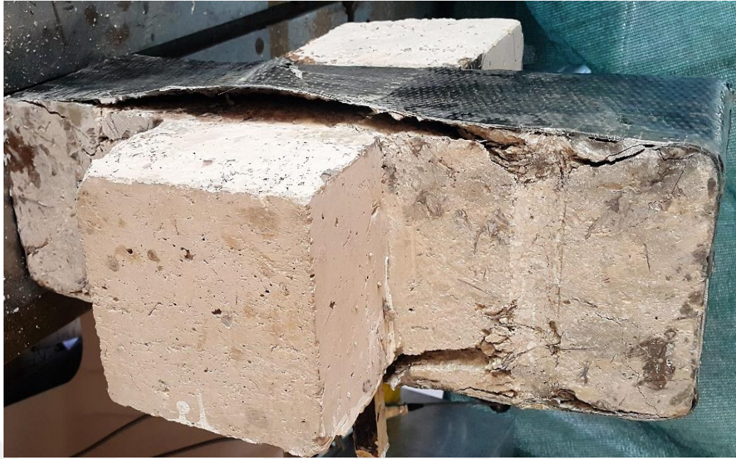
Figure 4.54 Specimen (C18-1.0-750 ) de-bonding failure after strengthening
