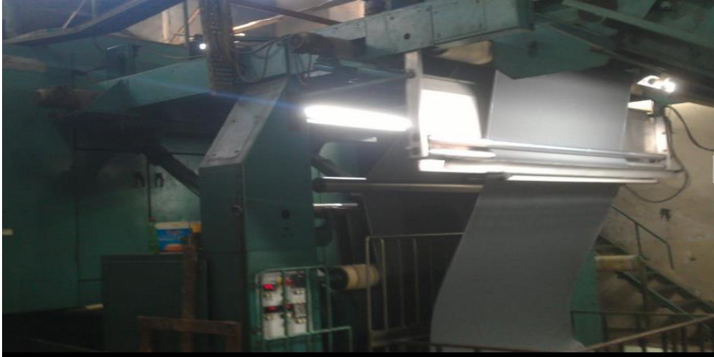
Figure 6.14 Chemical finishing (photo taken by the author)
