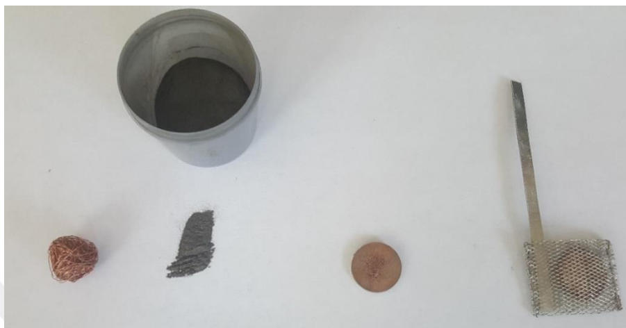
Figure 3.1 Photograph showing the preparation of electrodes from Cu wire matrix and powders. The prepared electrode is enveloped in a Ni mesh.
