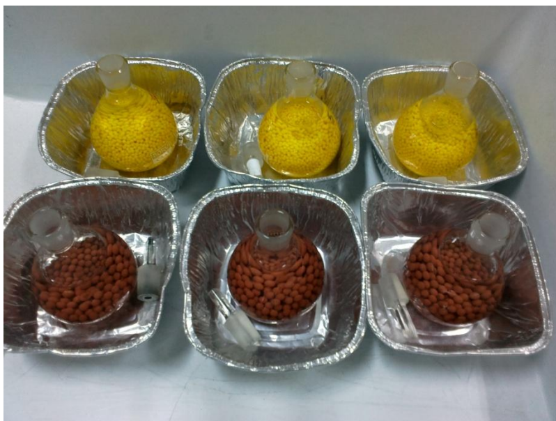
Figure 2.11 Density measurement using water displacement method
