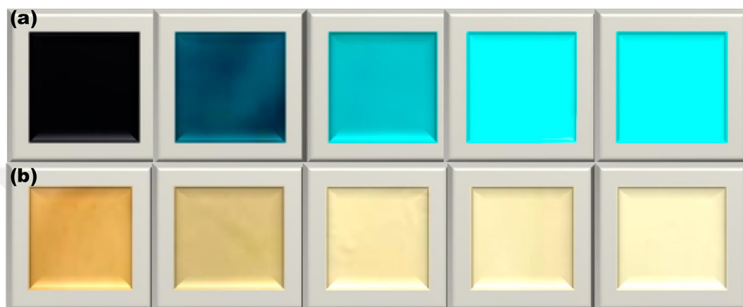
Figure 6.30: Visual colorimetric detection of TNT. Photograph of the fluorescence quenching of FNFM treated with different concentrations of TNT in aqueous phase when viewed under UV ( \lambda_{\text{ext}}=254\text{ nm} ) a) and daylight b). The tested TNT concentrations are 5 \times 10^{-3} , 5 \times 10^{-4} , 5 \times 10^{-5} , 5 \times 10^{-6} , and 5 \times 10^{-7}\text{ M} from left to right.
