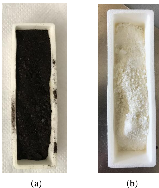
Figure 4.12 : (a) before and (b) after calcination step sample's view.
