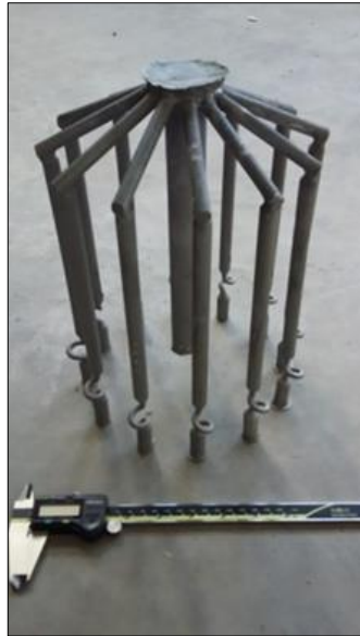
Figure 3.5: Bunches of specimens after casting process.
