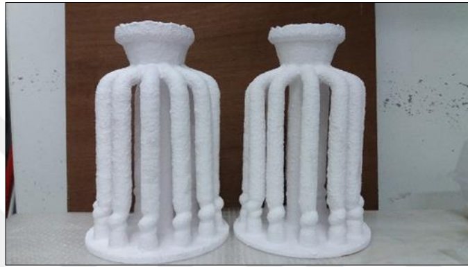
Figure 3.2: The moulds after baking process.
