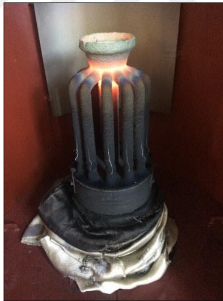
Figure 3.4: A mould after casting process.
