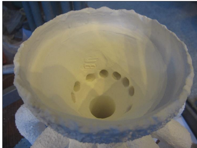
Figure 3.3: The gating system of the moulds.
