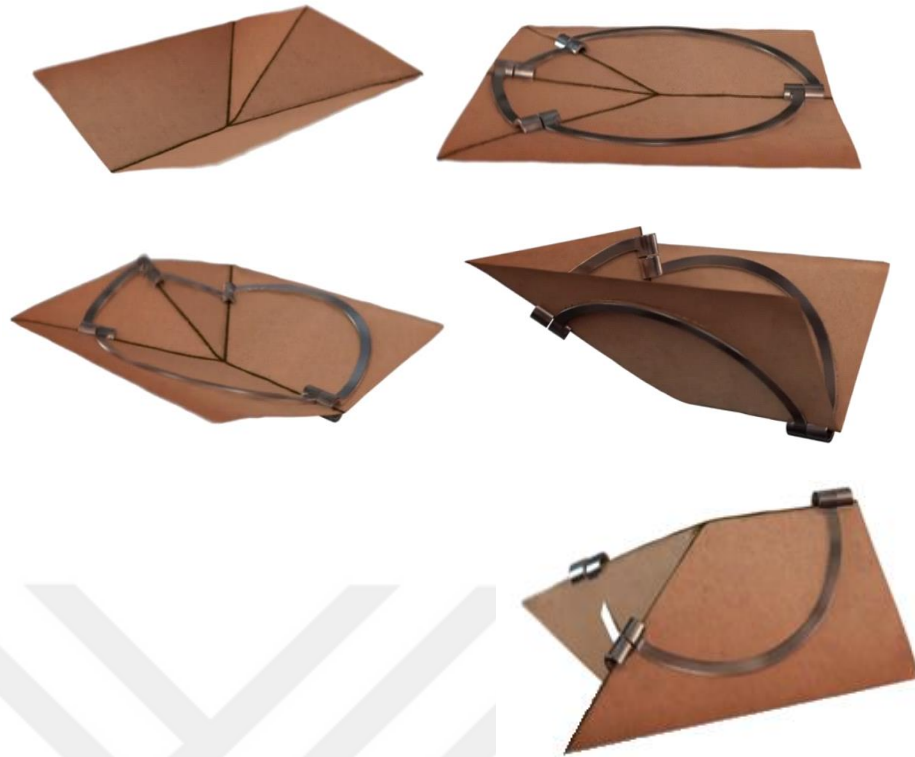
Figure 48 Miura-Ori Unit as a Spherical Mechanism (Source: Mooth, 2014.)
