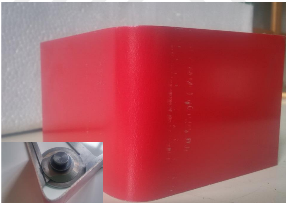
Figure 6.3 Cold Bent Specimen with Angle of 75°
