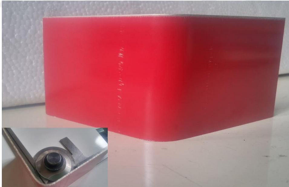
Figure 6.1 Cold Bent Specimens with Angle of 90^{\circ}
