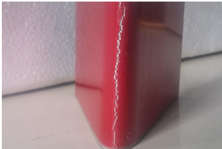
Figure 6.7 Cold Bent Specimen with Angle of 45°
