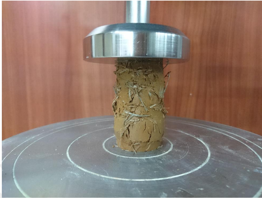
Figure 4.18. Unconfined compression test specimen of AC-03 mixture after the testing process
