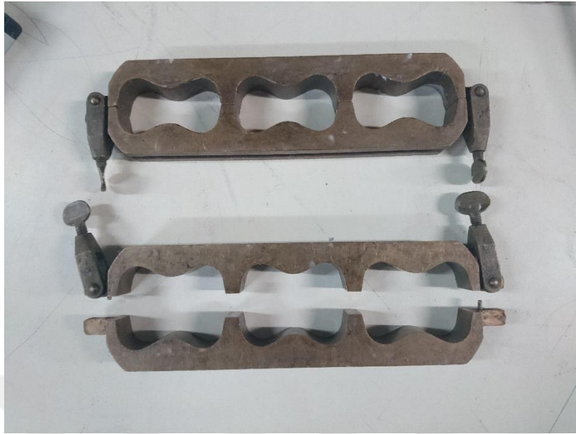
Figure 3.24. Compaction mold which was used in this study to prepare 8-shaped specimens
