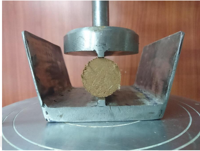
Figure 4.13. Indirect split tensile test specimens with synthetic fiber content before testing process
