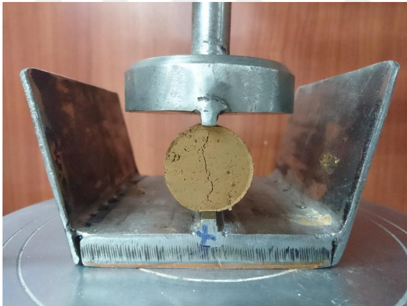
Figure 4.12. Indirect split tensile test specimens with metal swarf content after testing process
