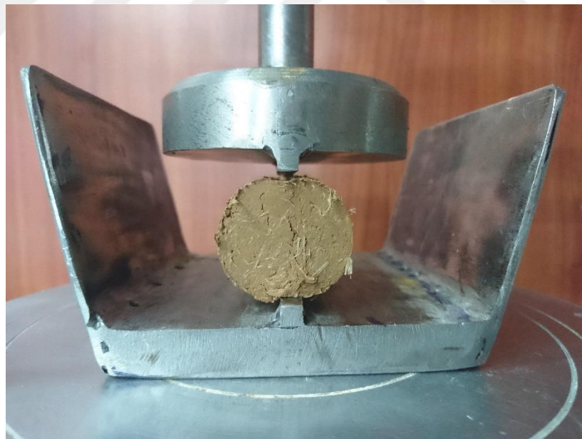
Figure 4.14. Indirect split tensile test specimens with synthetic fiber content after testing process
