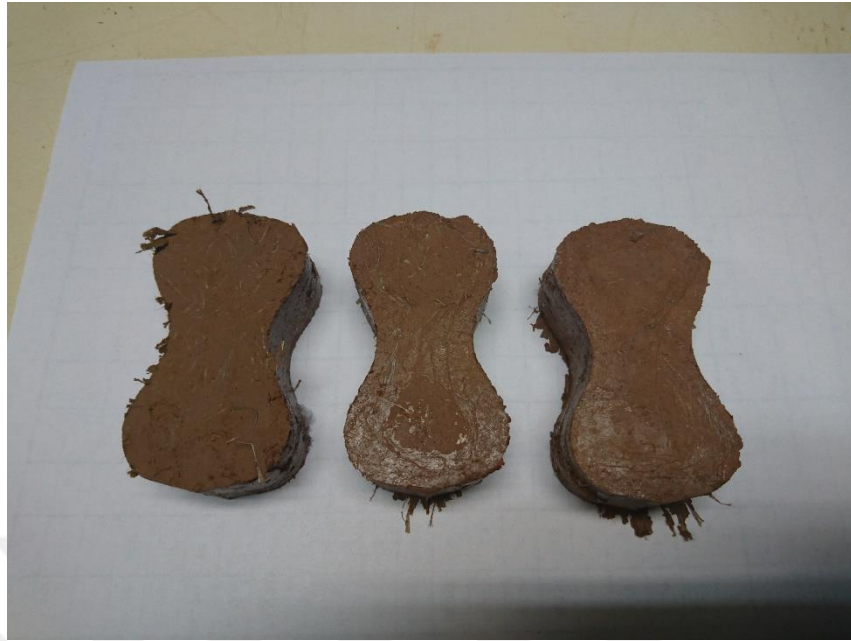
Figure 4.6. 8-shaped direct tensile test specimens with synthetic fiber content before testing process
