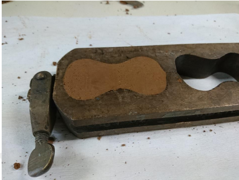
Figure 3.26. Specimen after compaction process in the mold
