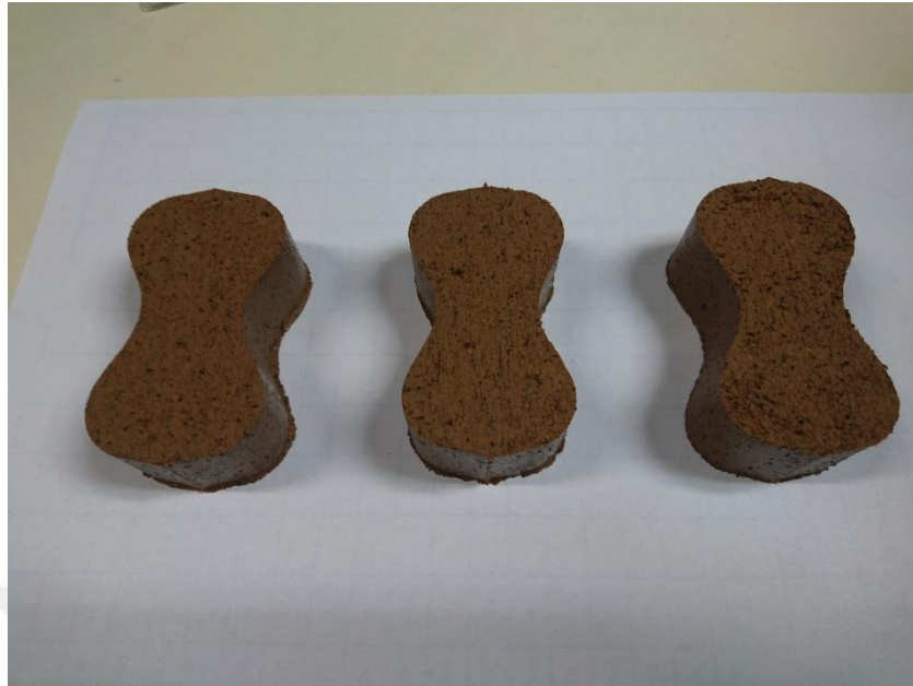
Figure 4.2. 8-shaped direct tensile test specimens with pulverized rubber content before testing process
