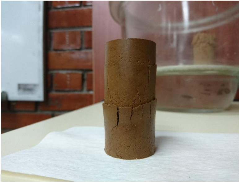
Figure 4.16. Unconfined compression test specimen of AC-01 mixture after the testing process
