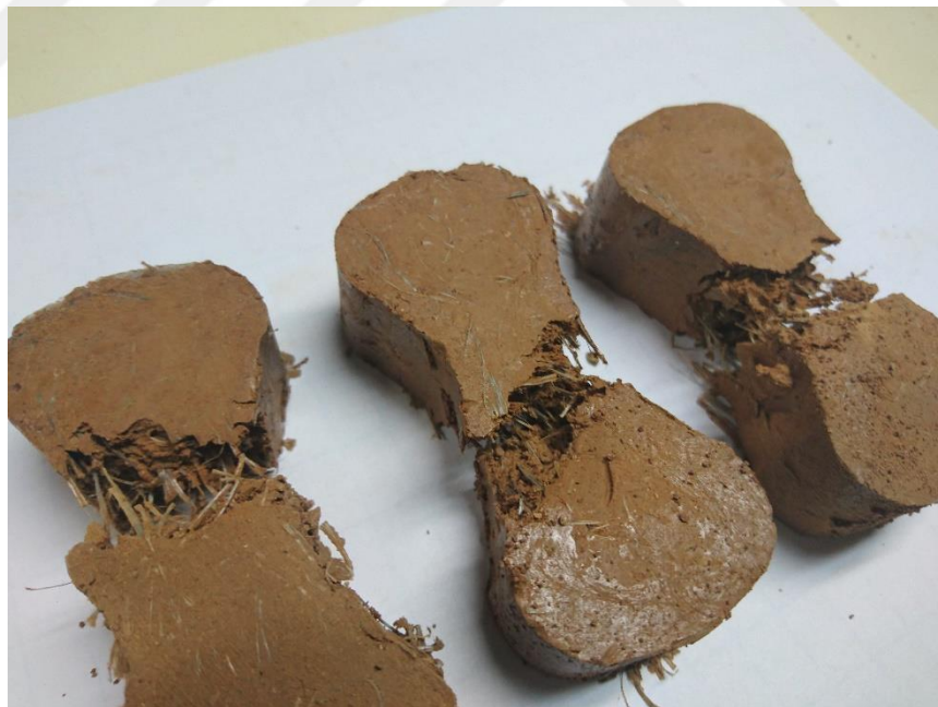
Figure 4.7. 8-shaped direct tensile test specimens with synthetic fiber content after testing process
