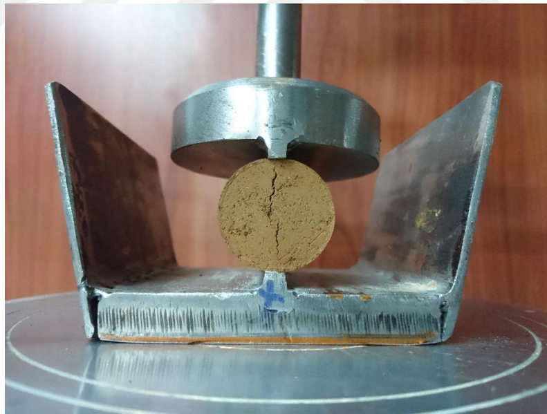
Figure 3.37. Split tensile test specimen after the testing process
