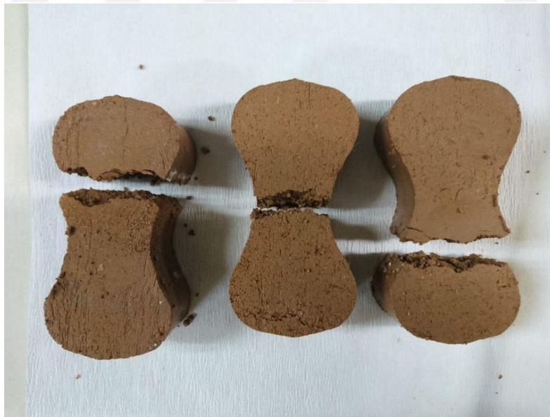
Figure 3.31. Tension failure of the 8-shaped specimens after direct tensile testing
