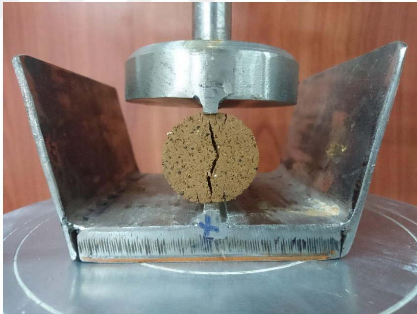
Figure 4.10. Indirect split tensile test specimens with pulverized rubber content after testing process
