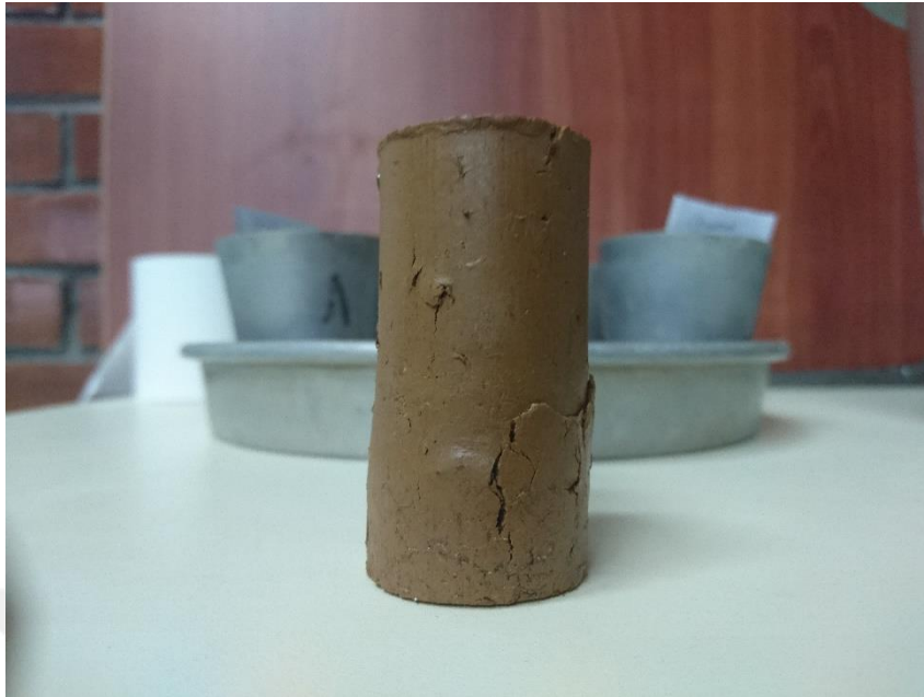
Figure 4.20. Unconfined compression test specimen of AC-06 mixture after the testing process
