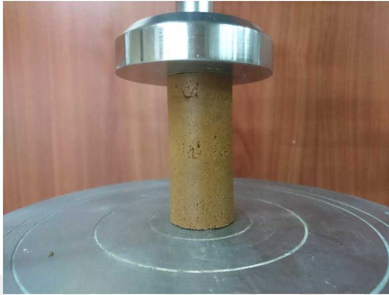
Figure 3.39. Unconfined compression test specimen before testing process
