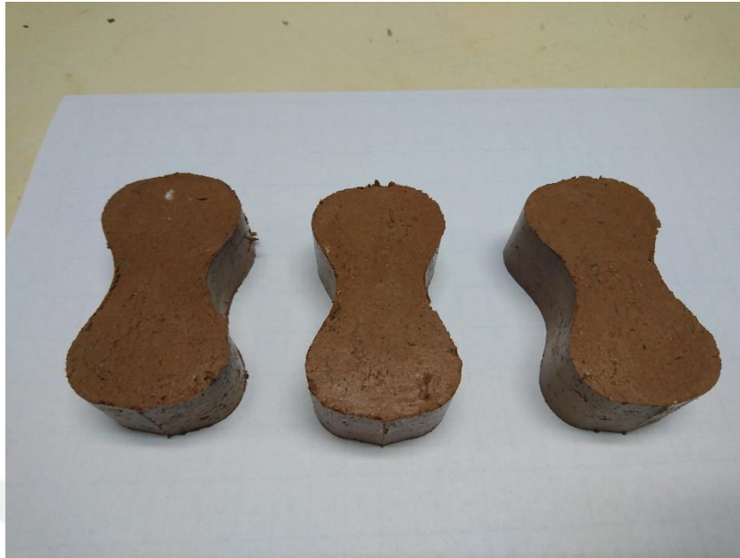
Figure 4.4. 8-shaped direct tensile test specimens with metal swarf content before testing process
