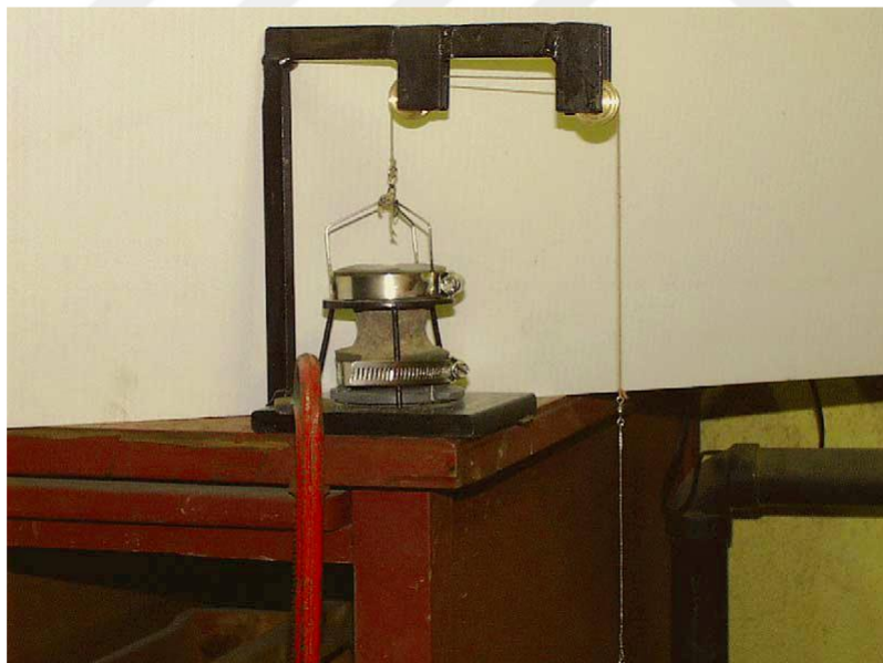
Figure 2.10. Direct tensile strength setup developed for sandy loam soil (Ibarra et al., 2004)
