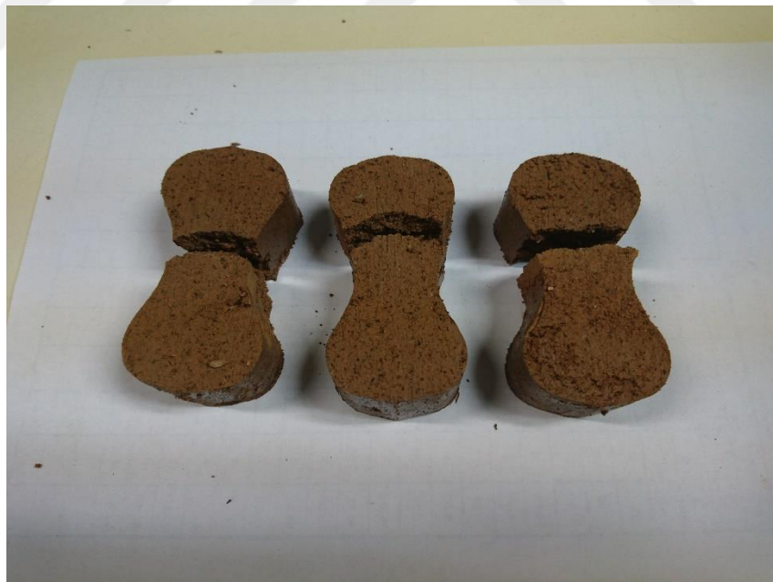
Figure 4.3. 8-shaped direct tensile test specimens with pulverized rubber content after testing process
