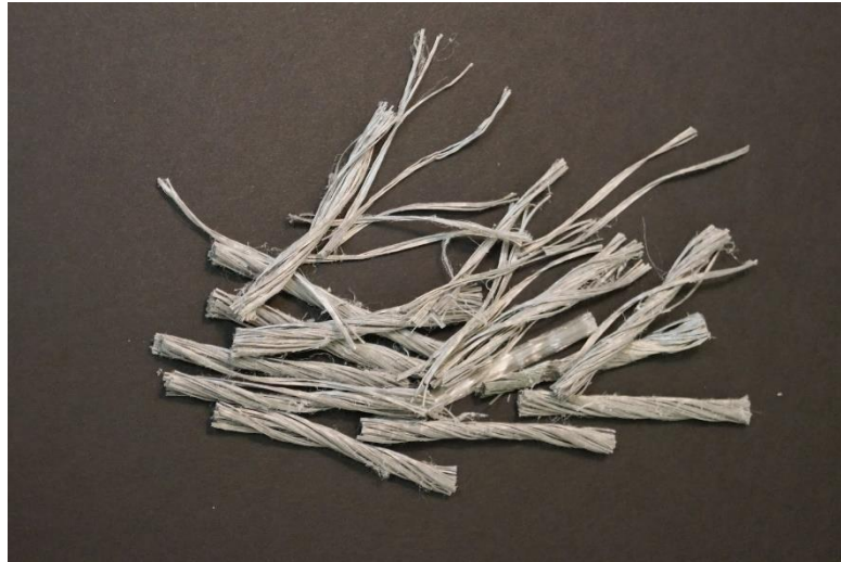
Figure 2.26. An example of polypropylene fiber which is used for tensile strength stabilization and improvement (Adopted from www.fortaferro.com )
