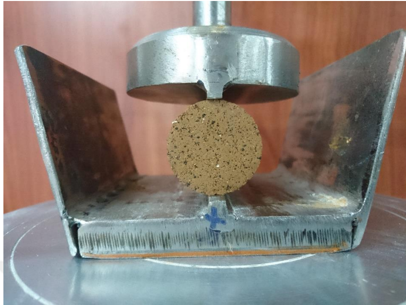
Figure 4.9. Indirect split tensile test specimens with pulverized rubber content before testing process
