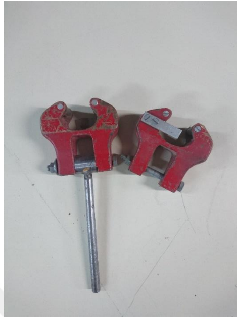
Figure 3.30. Grips which were used to place 8-shaped soil specimen for direct tensile testing
