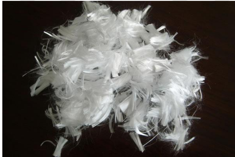
Figure 2.27. An example of polyester fiber which is used for tensile strength stabilization and improvement (Adopted from www.polyrope-fence.com )
