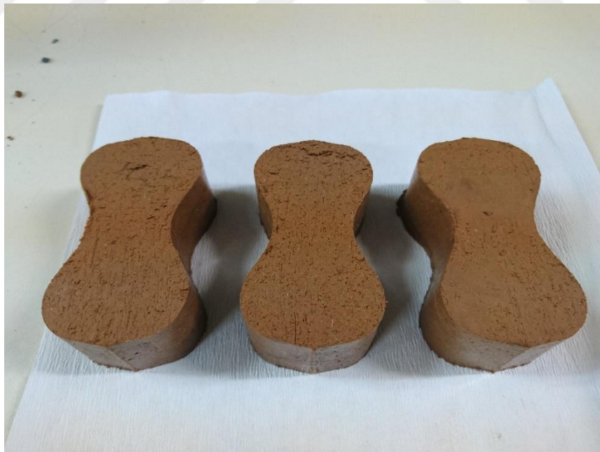
Figure 3.27. Compacted and extracted soil specimens for direct tensile testing
