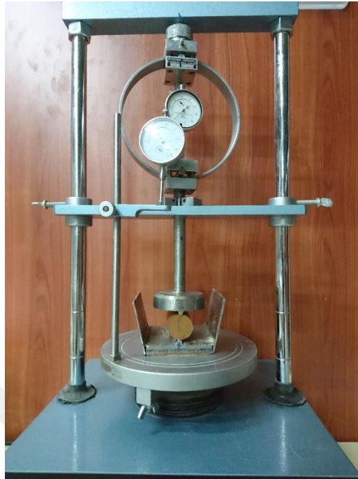
Figure 3.34. An overview of split tensile test with unconfined compression test machine
