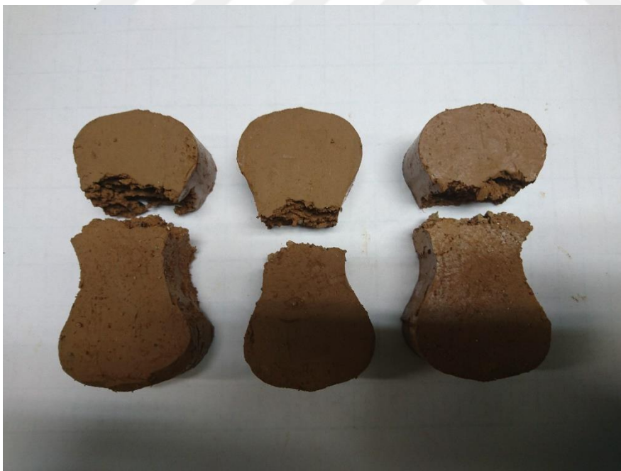
Figure 4.5. 8-shaped direct tensile test specimens with metal swarf content after testing process
