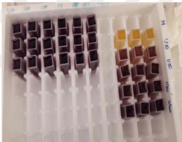
Figure 3.4. Preparation of standard DPPH solutions to obtain calibration curve
