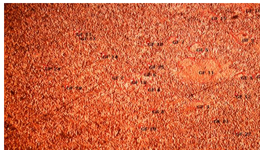
Figure 51. The samples recrystallized at 730°C for 150, 180, 210min respectively and aged at 450°C for 90min
