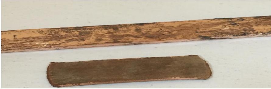
Figure 14. CuNiSi alloy slab after solidification
