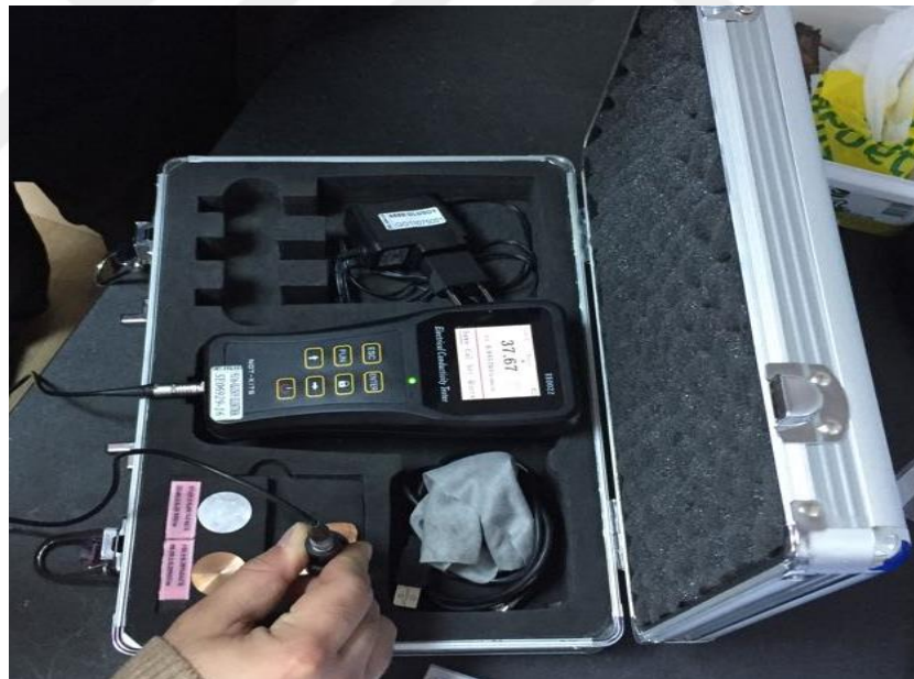
Figure 28. Electrical conductivity test device used for IACS% measurements
