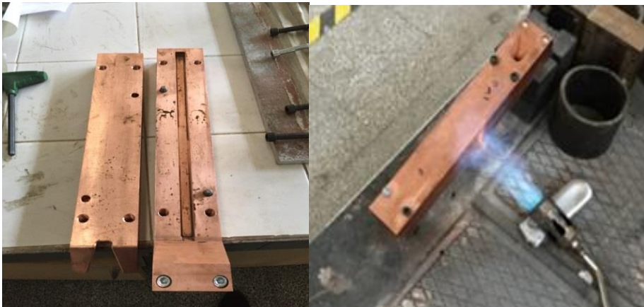
Figure 15. Permanent molds made of pure Copper during preheating
