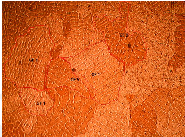
Figure 29. Cast microstructure of CuNiSi alloy
