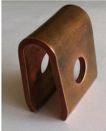
Figure 27. Picture of 180 o bent CuNiSi alloy sample specimen which will be used as catenary grip
