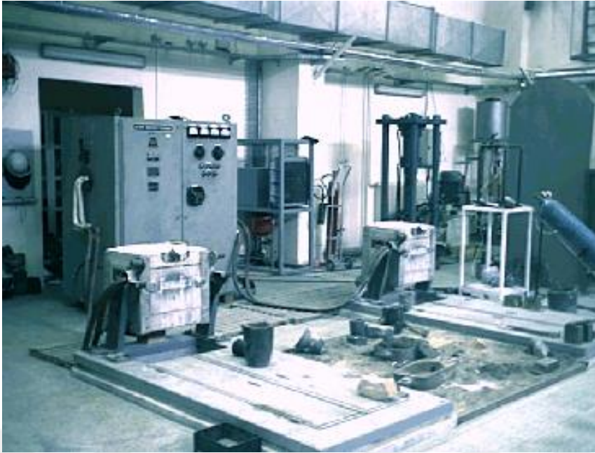
Figure 18. Induction furnaces used in this study
