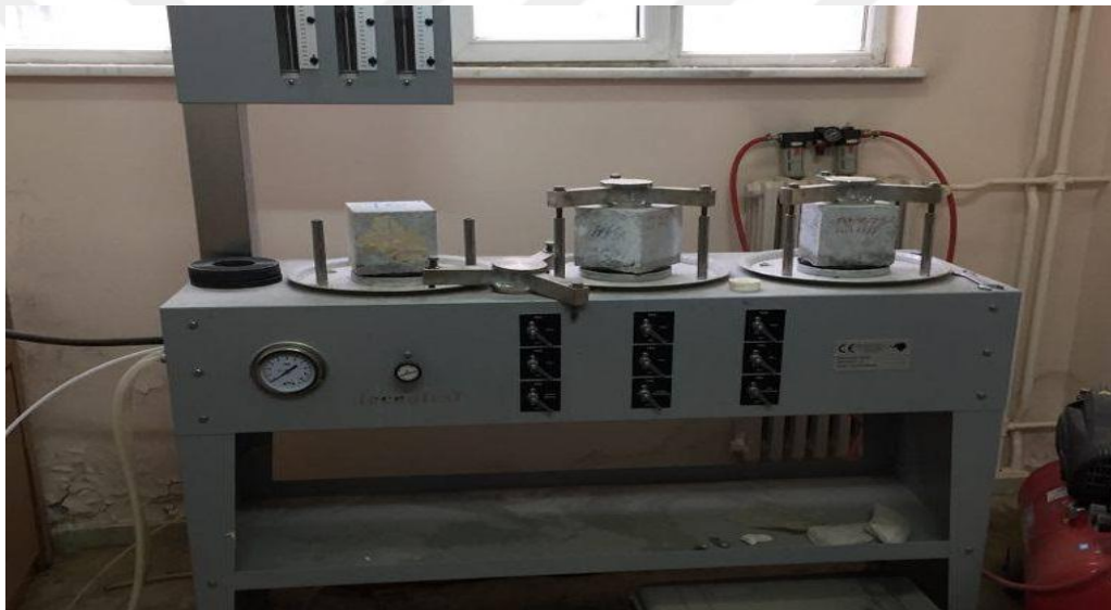
Figure 3.6 Water permeability test set up
