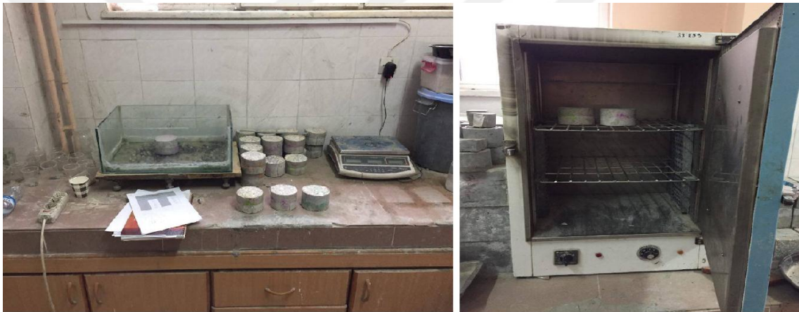
Figure 3.2 Photos of water sorptivity measurement
