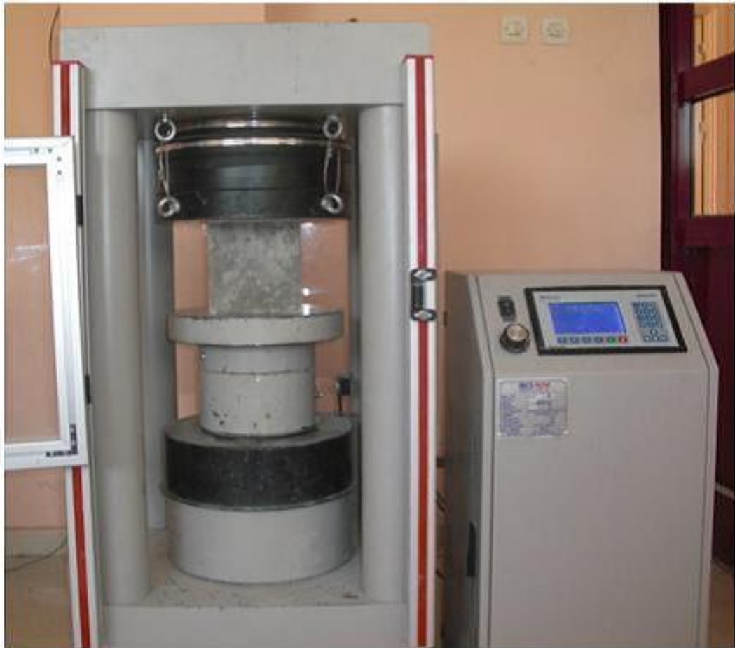
Figure 3.8 Compressive strength test
