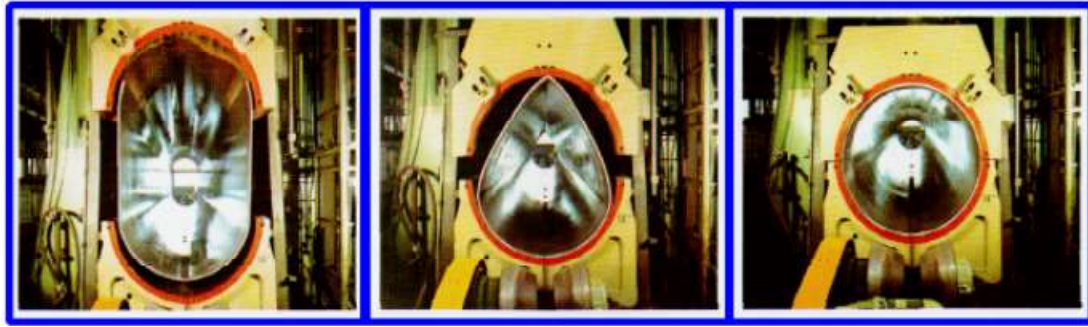
Figure 1.5 Forming of large CHS [6]
