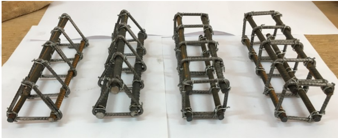
Figure 4.1 Rectangular and equilateral triangle steel bar reinforcement
