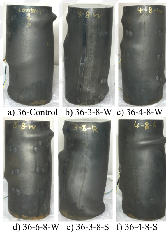
Figure 5.29 Failure mode of 3.15 thickness steel tube specimens with \phi 8 mm reinforcing bars
