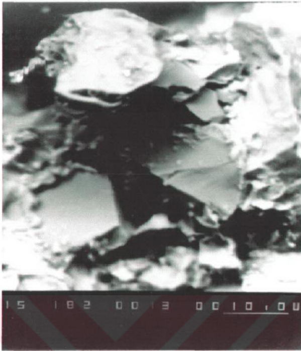
Figure 5. 2 Fracture surface for the isothermally tested at 430 °C AlSi7/SiC/20 p composite showing the void formed at the cracked particle and expanding into the matrix.
