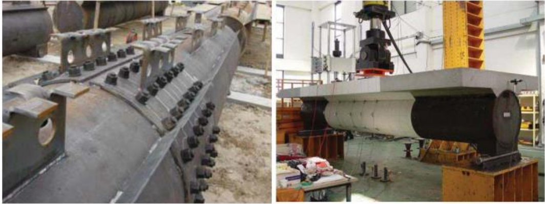
Figure 2.6 Bolt connections of specimen
