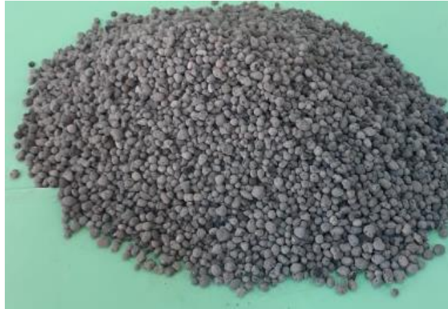
Figure 3.3 Clay aggregate (LECA)
