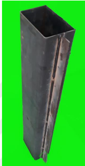
Figure 3.4 Welding process of steel tube
