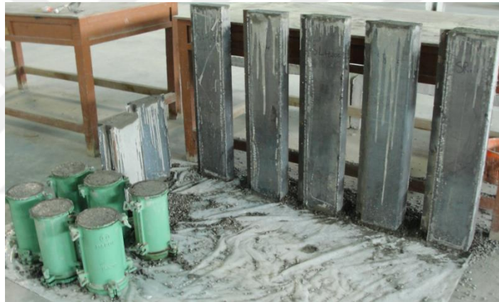
Figure 3.6 Casting the LWC inside the steel tube
