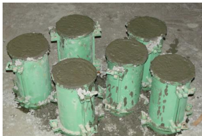
Figure 3.7 Molds after casting
