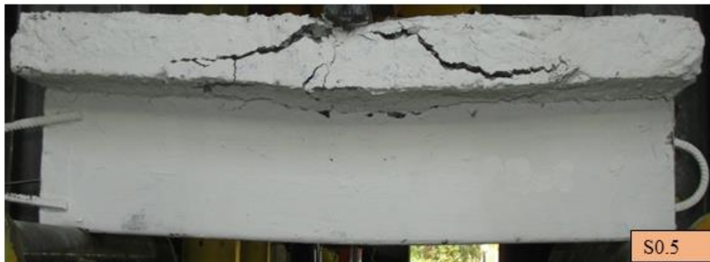
Figure 4.3 Cracks for the testing specimens
