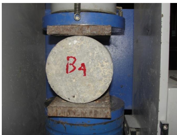
Figure 3.11 Splitting tensile strength test
