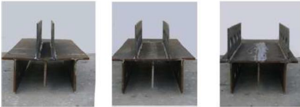
Figure 2.8 Details for push out tested specimens
