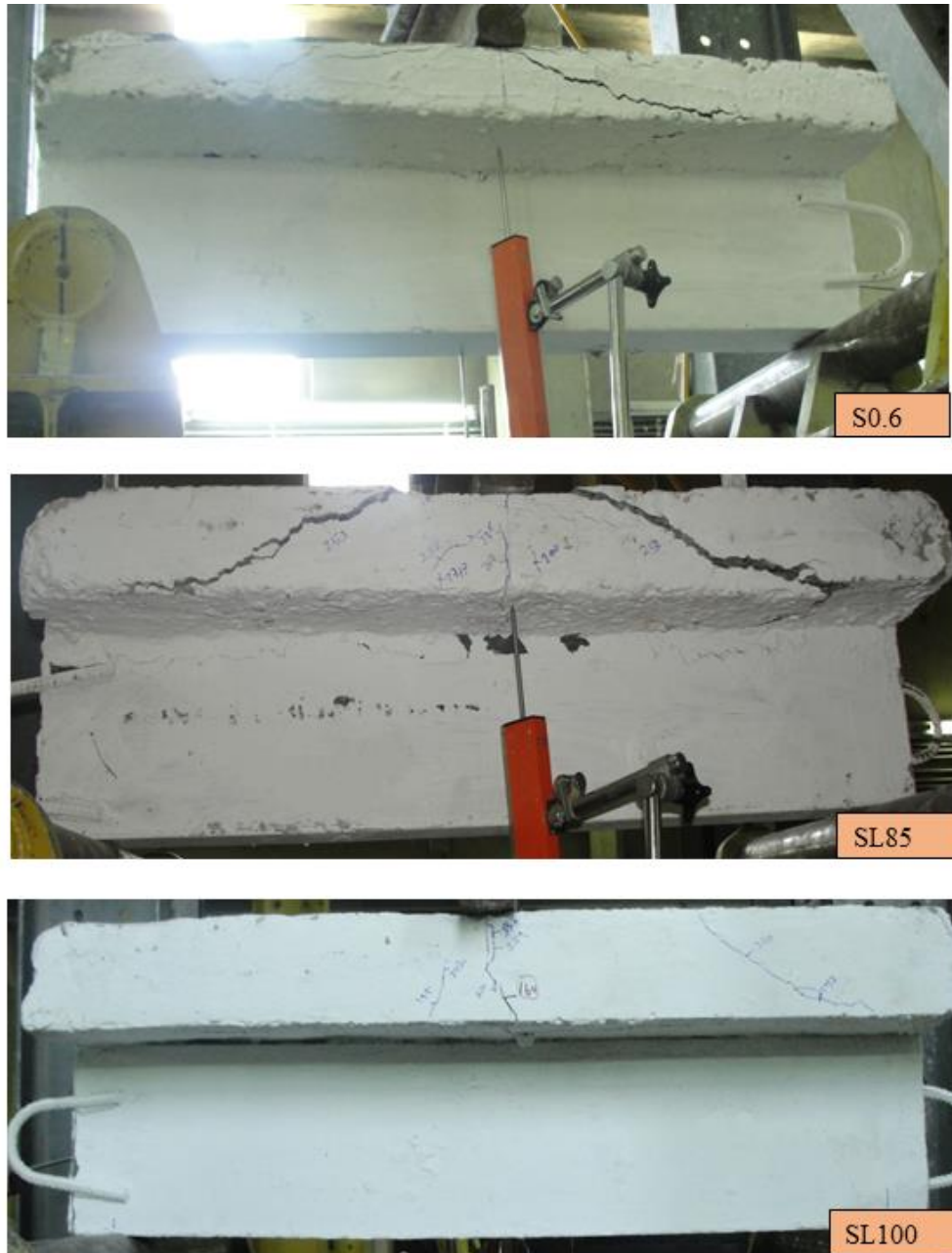
Figure 4.4 Cracks for the testing specimens
