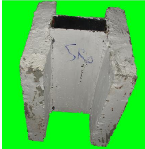
Figure 3.17 Hollow steel tube and typical composite H beam specimen
