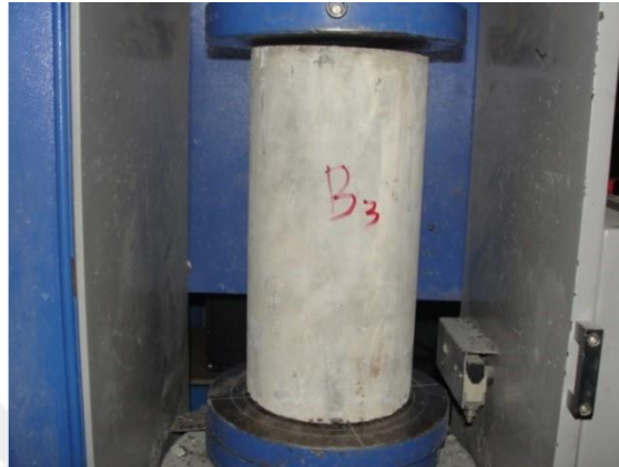
Figure 3.10 The compressive strength instrument
