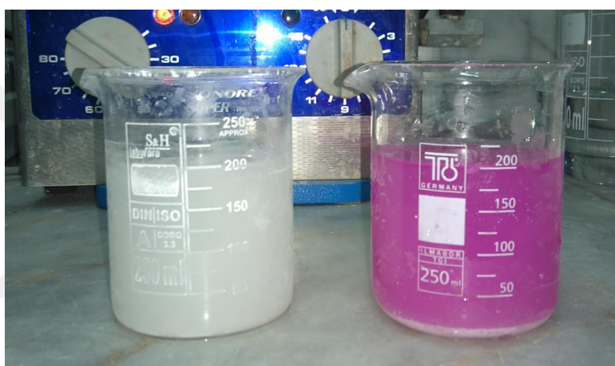
Figure 3.8. The colors of citric acid solution containing calcined magnesia sample with phenolphthalein indicator at the beginning (left) and at the end (right) of the reaction.
