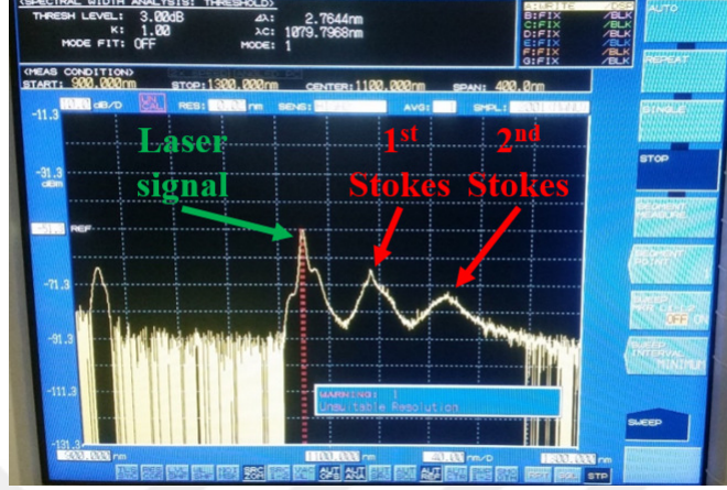
Figure 1.7: An optical spectrum example with Stokes emissions due to the SRS.
