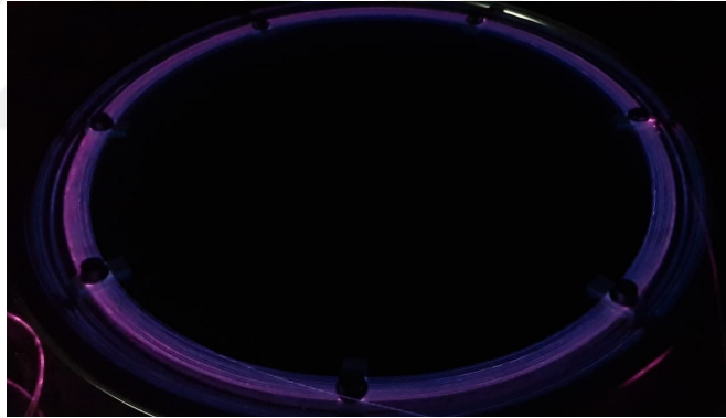
Figure 3.16: The photograph of fiber coiling system, having 1 m diameter, taken with a cell phone while the laser is on showing the fluorescence in blue region.
