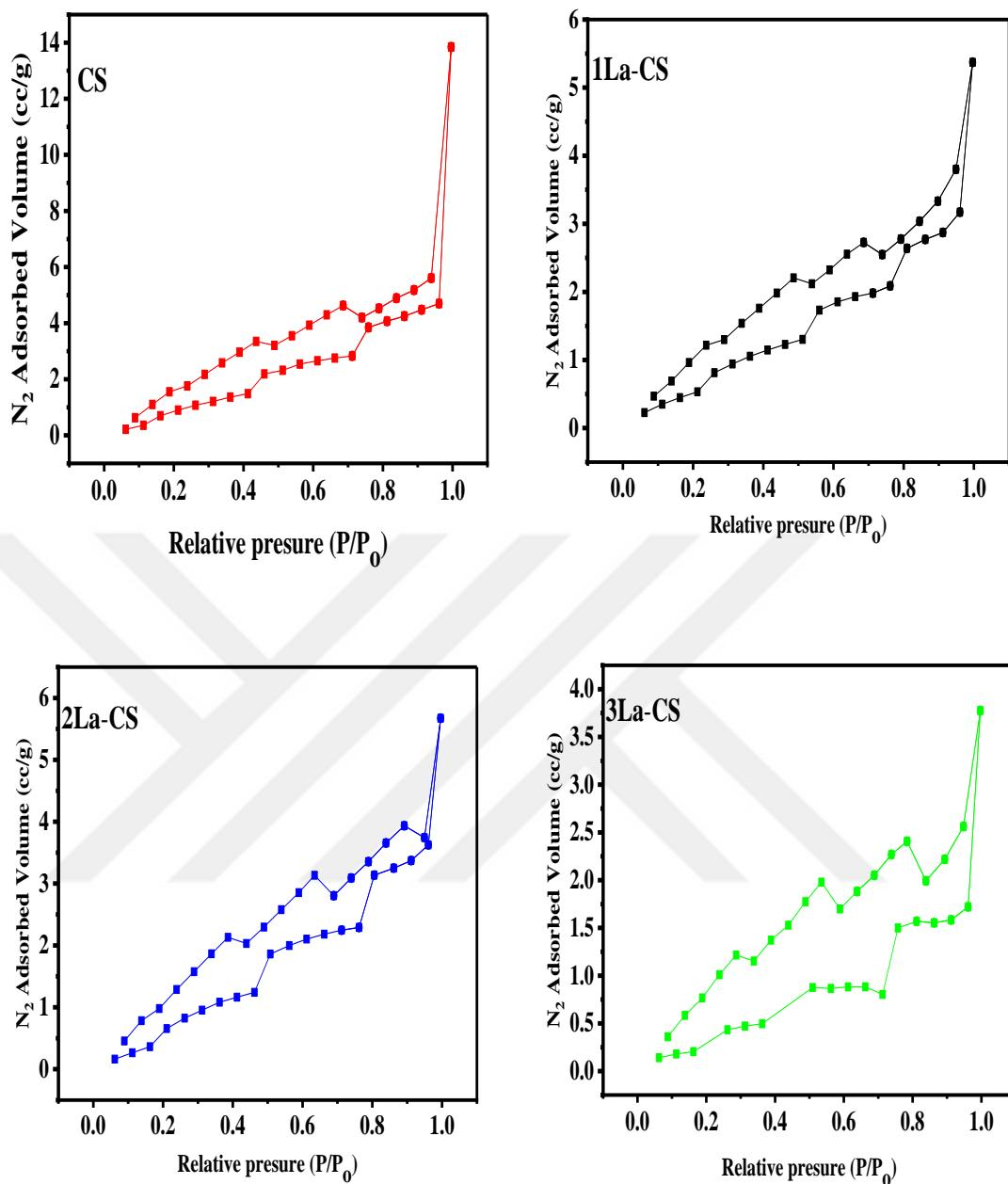
Figure 4.5.  $N_2$  adsorption-desorption isotherm.
