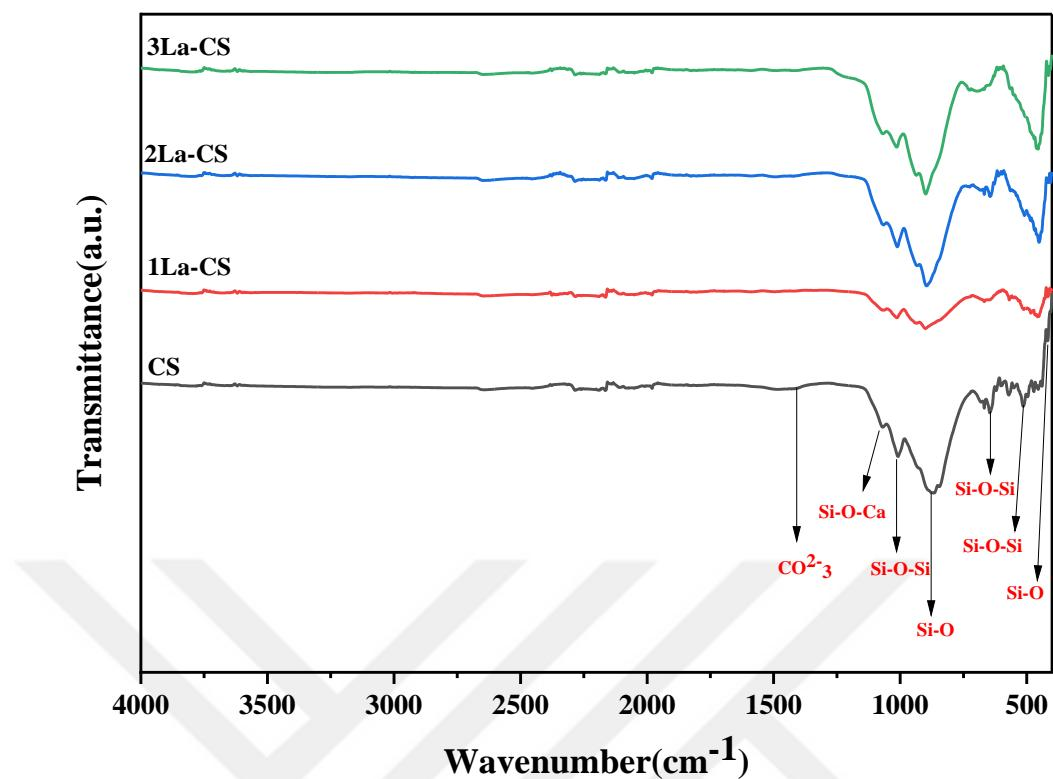
Figure 4.2. FTIR spectra of CS and La-CS materials calcined at 900°C for 2h.
