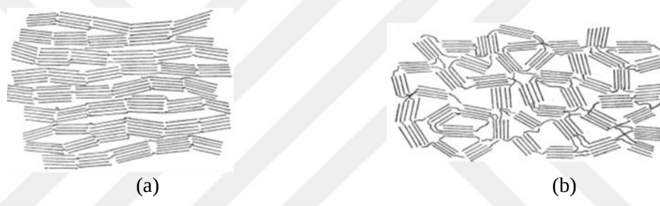
Figure 2.8. Scheme representation of AC structure: (a) graphitized carbon, and (b) non-graphitized carbon [109]
