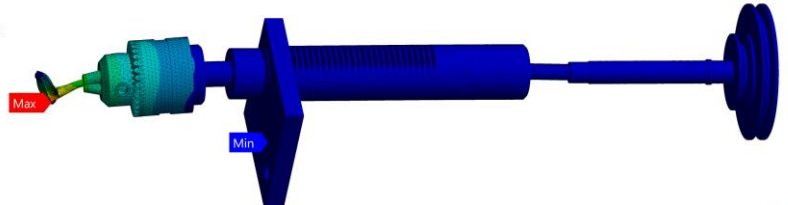
G: 50mm 4340 Transient Structural Total Deformation Type: Total Deformation Unit: mm Time: 1
