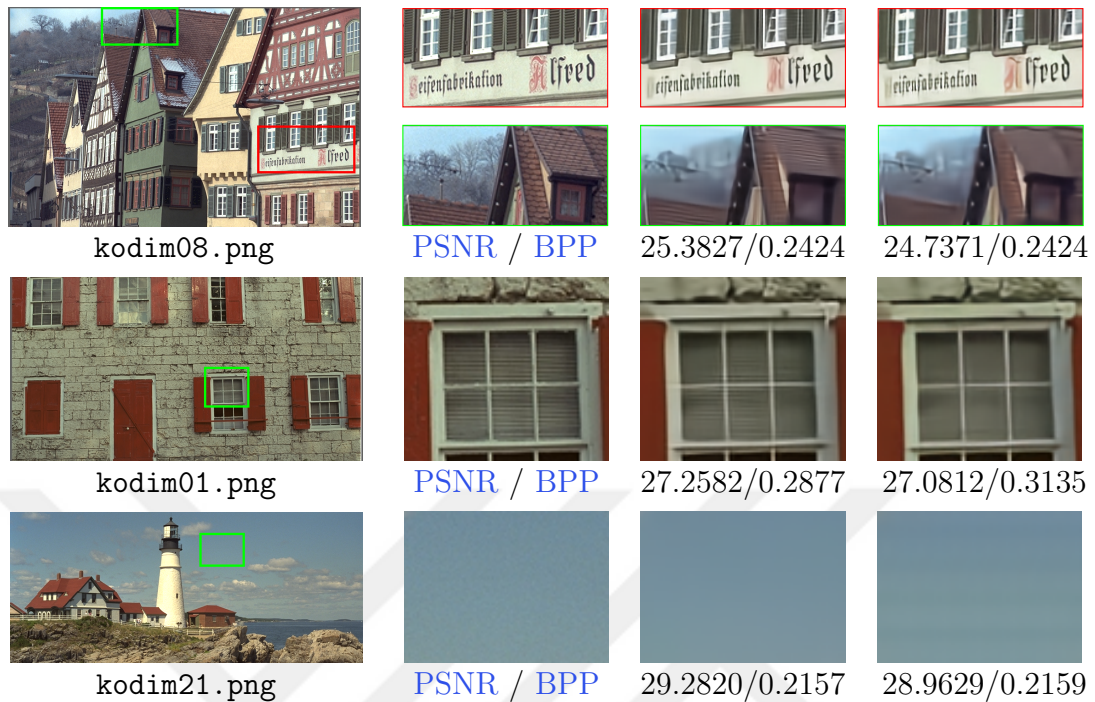
Figure 5.9: Visual evaluation of reconstructed kodim08.png , kodim01.png and kodim21.png images, respectively, in Kodak dataset. Crops are taken from ground truth, PadéNet version of joint autoregressive network with GDN, and original joint autoregressive models, respectively. For kodim08.png , the crops are taken from the models trained with \lambda = 0.0018 , and the others are taken from the models with \lambda = 0.0035 in the rate-distortion loss.
