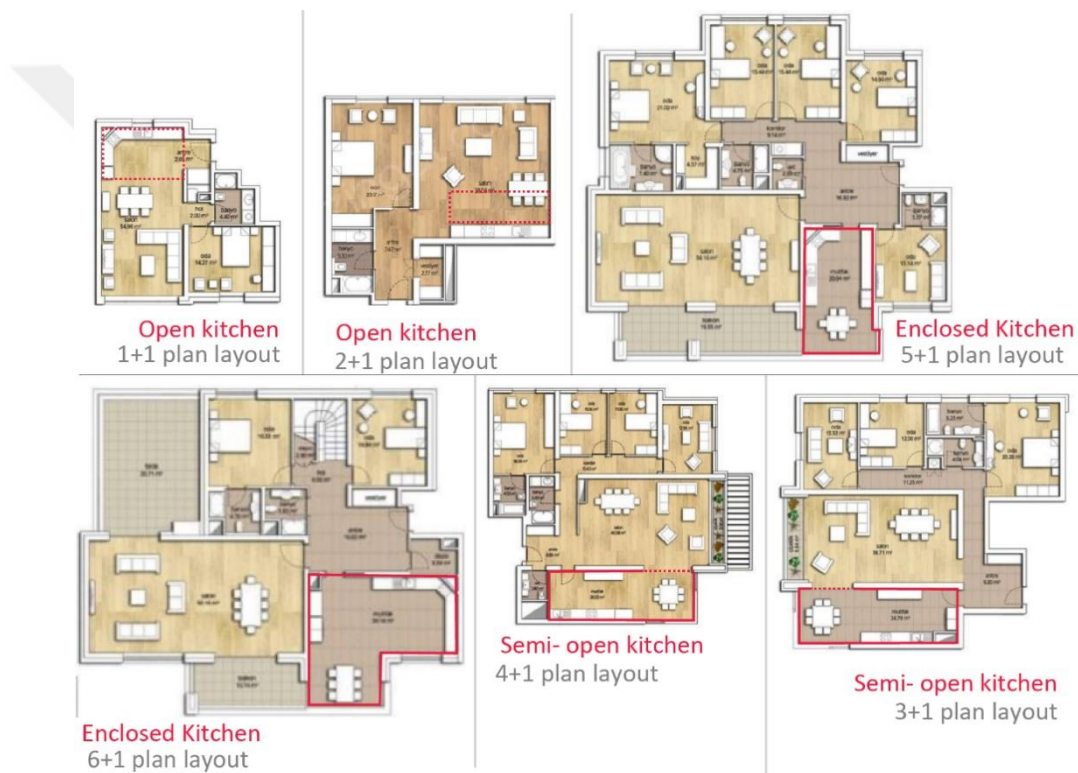
Figure 12. Floor plans of apartment flat types in Park-Oran Housing (Adapted from Kale, 2008)
