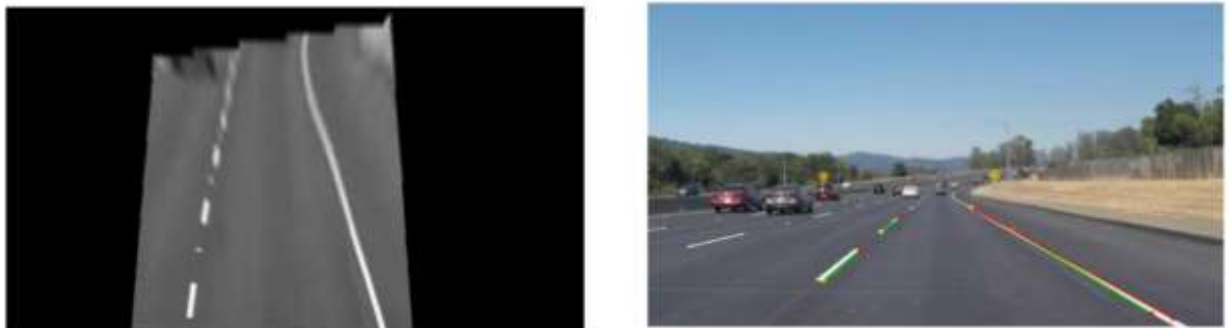
Figure 4.4: Binarizing for Yellow (Left) and White (Right) RGB Thresholds.
