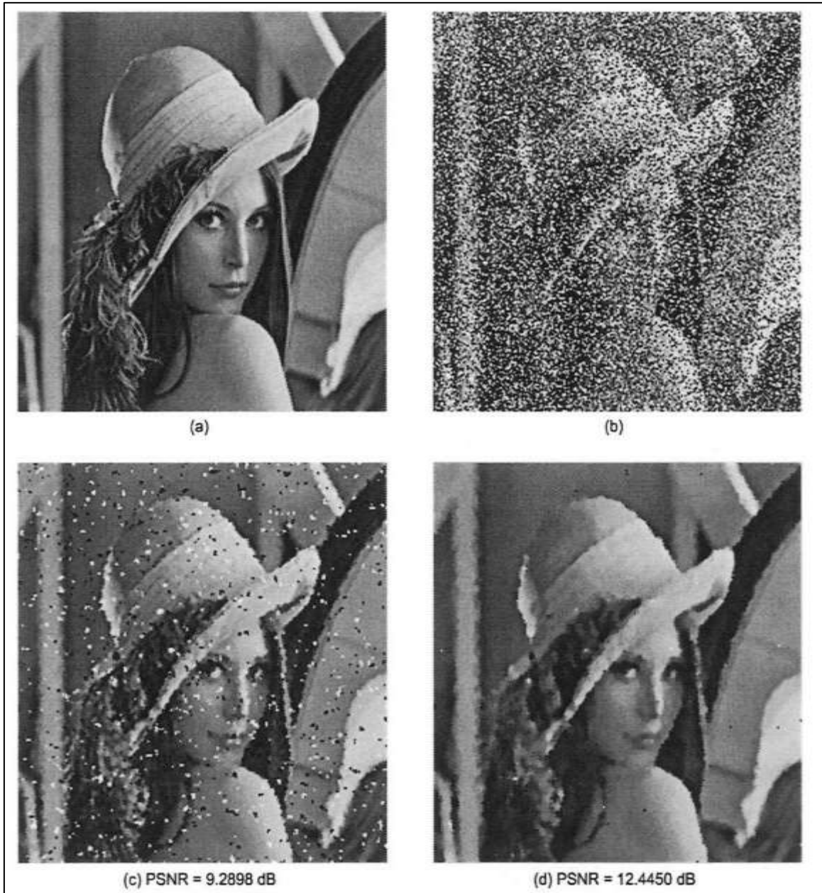
Figure 3.6: The Application of Nonlinear Filtering [5].
