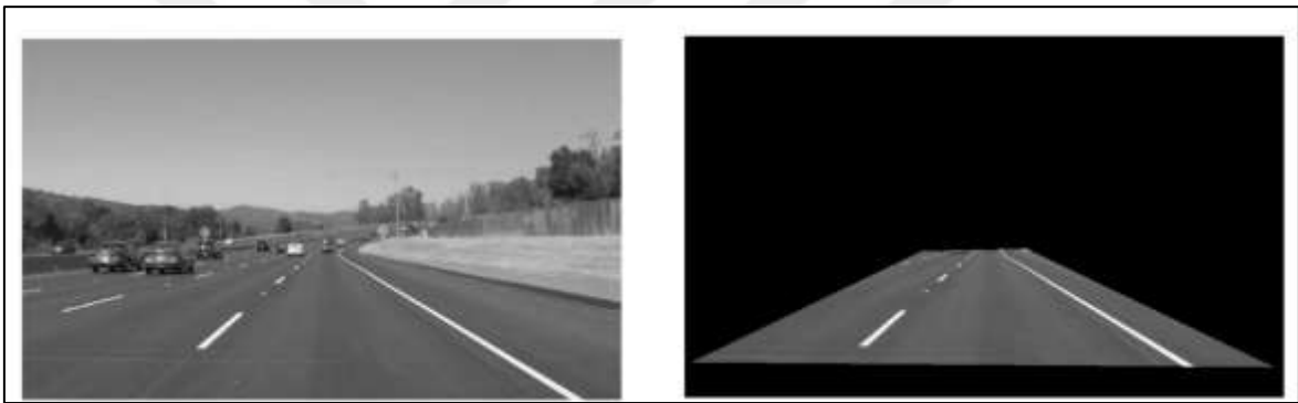
Figure 4.3: First Frame of the Video (Left) Is Processed to the Gaussian Filtered Frame (Right).
