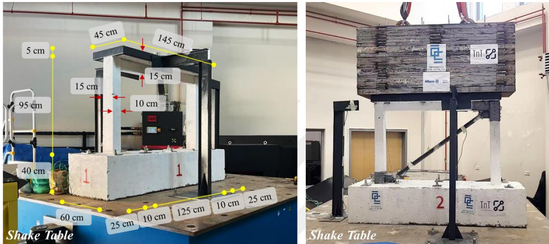
Figure 3.4 : Shake table test setup for two specimens.
