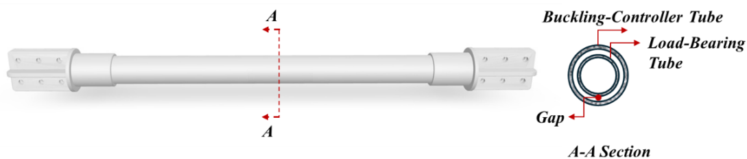
Figure 4.2 : Schematic representation of a Tube-in-Tube buckling restrained brace.
