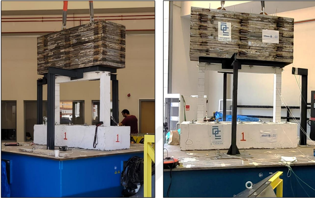
Figure 2.6 : Specimen on the shake table.
