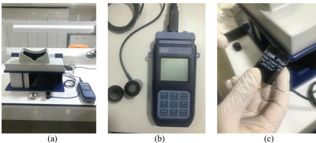
Figure 44: a) UV Cabin b) Photo-radiometer and c) One of the sensors used in the procedure.
