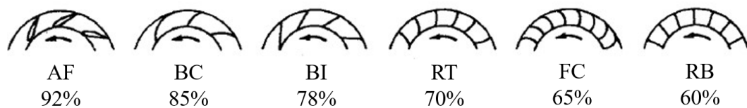
Figure 1.3 : Six blade shapes commonly used in centrifugal fans [5].
