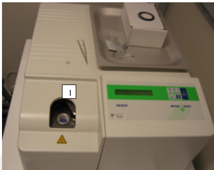
Figure 5.13 Differential Scanning Calorimeter (1) Sample Holder
