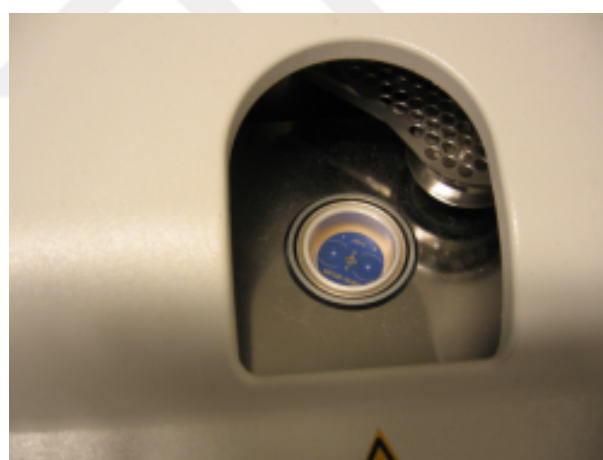
Figure 5.14 b Differential scanning calorimeter sample and reference holder
