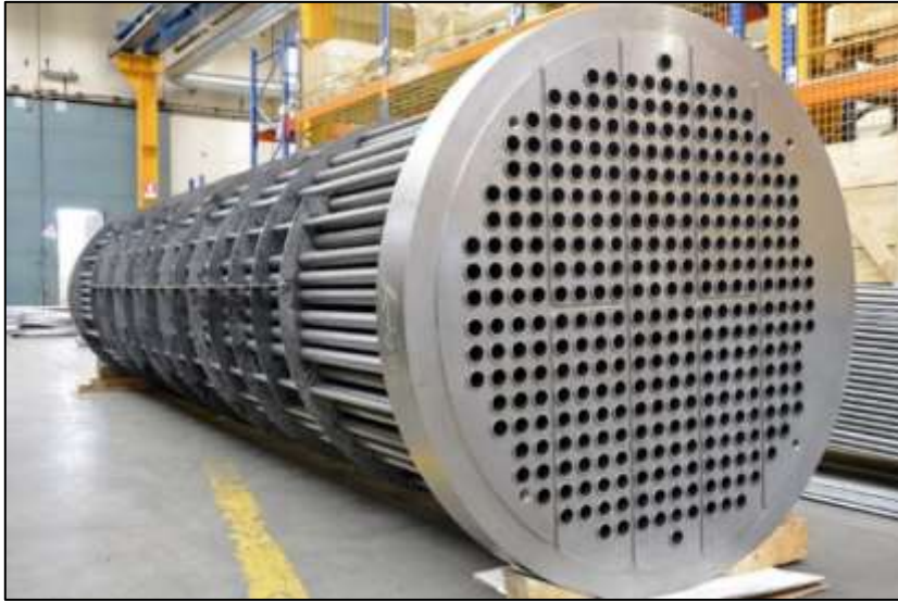
Figure 2.3: An Example of a Fixed Tube STHE [19].
