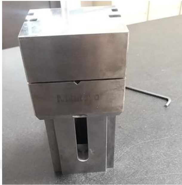
Figure 35 Mitutoyo Clamp to fix the Weld Plate
