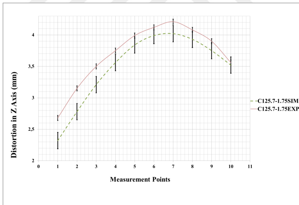
Figure 105 C 125.7-1.75 Simulation vs Experimental Distortion Comparison
