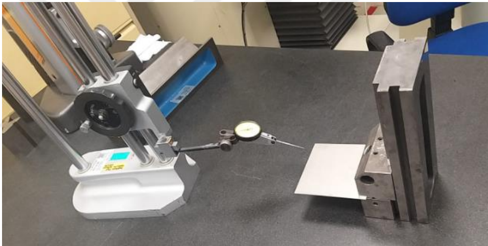
Figure 42 Measurement with Height Gauge Equipment
