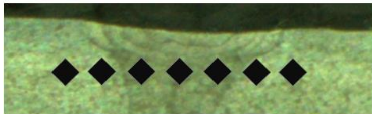
Figure 36 Hardness Test Points from Weld Plate after Welding Complete
