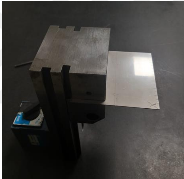
Figure 32 Fixture used in Welding Operation
