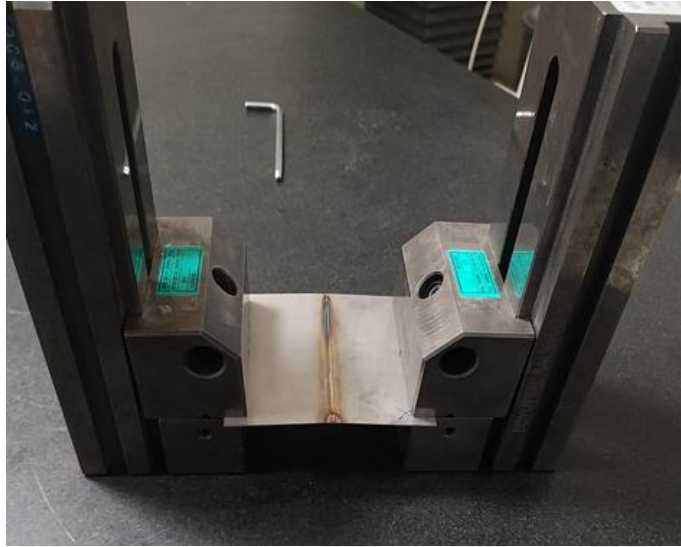
Figure 33 C 125.7-1.75TSC Specimen Fixture used in Welding
