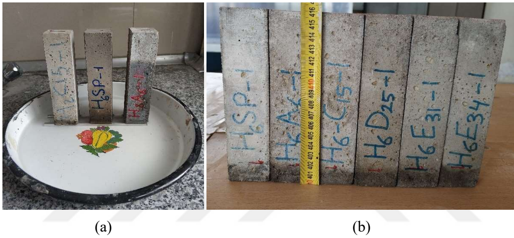
Figure 2. 10 (a) CWA test, (b) Measurement of the rise of water in the sample
