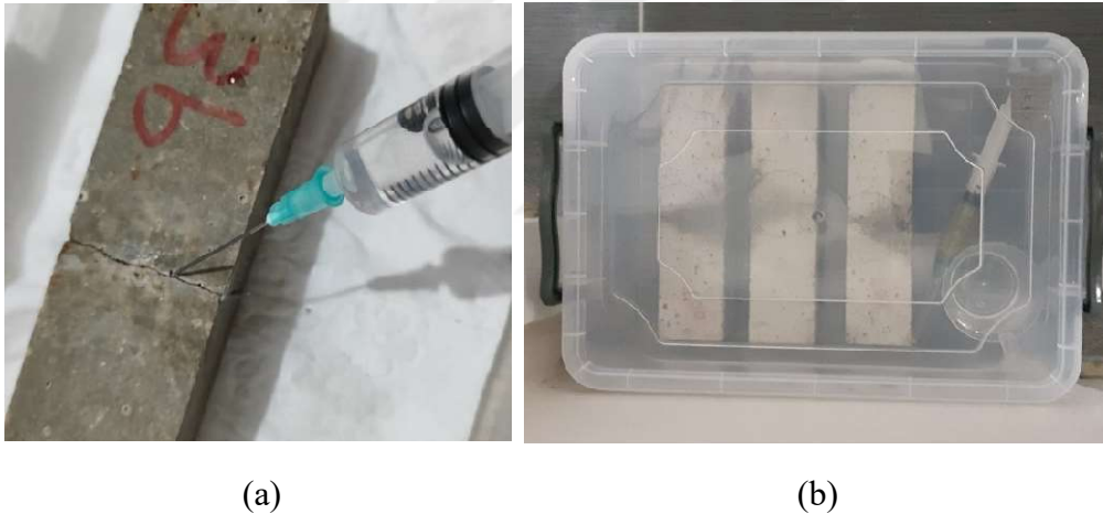
Figure 2. 7 (a) Healing the samples by injecting the bacteria, (b) Storing samples in special containers for each strain of bacteria
