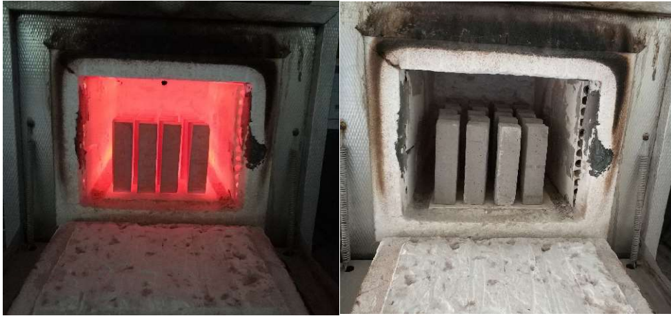
Figure 2. 5 Inducing cracks in H4, H6, and H8 samples by exposing to high temperature
