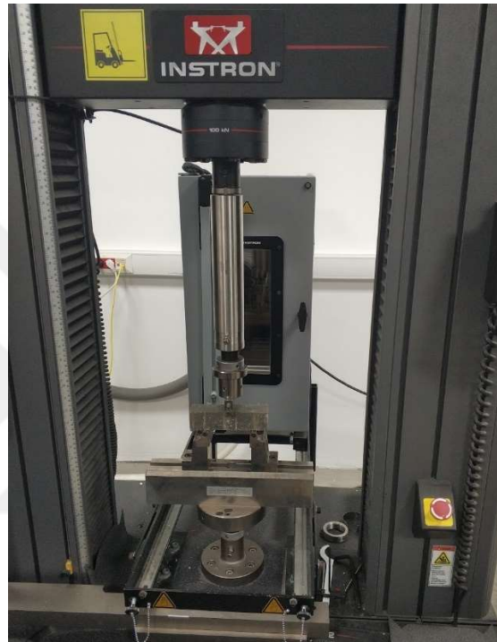
Figure 2. 4 Inducing crack in C and CB samples
