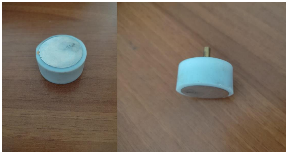
Figure 3.3. MgAZ61 substrate coated with GO/ZnO /Epoxy nanocomposite
