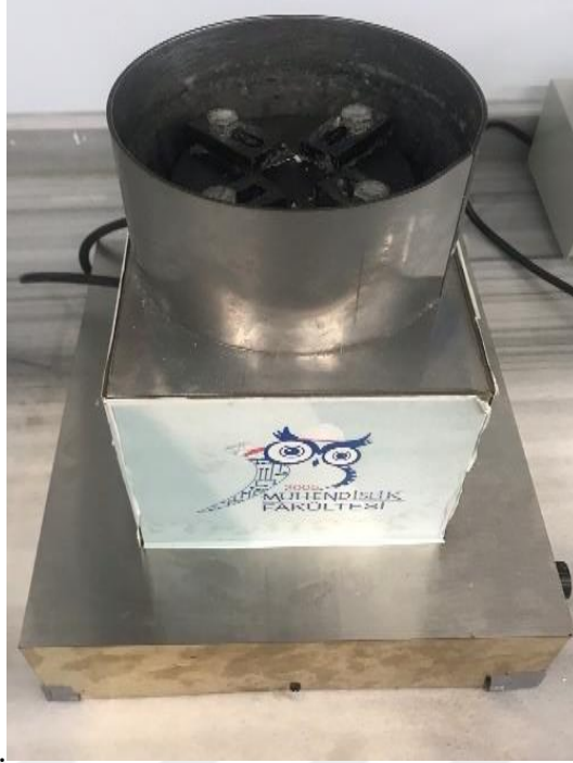
Figure 3.1. Spin coating device with maximum speed up to 1500 rpm
