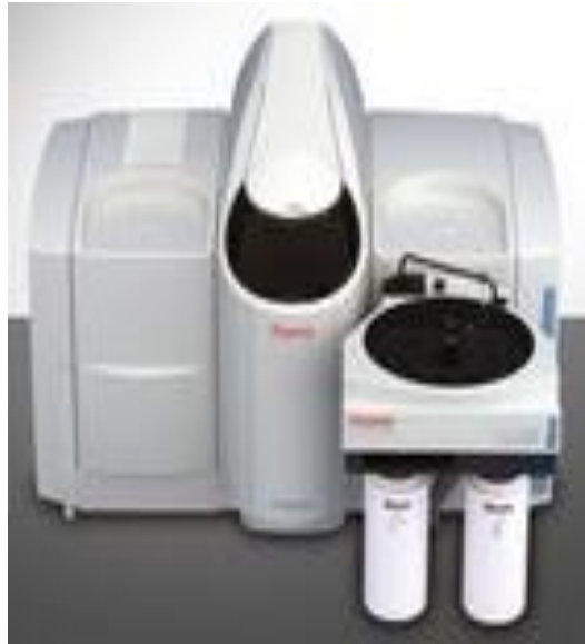
Figure 3.9. Fourier infrared transform spectroscopy device.
