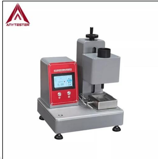
Figure 3.11. The device used to measure water contact angles.
