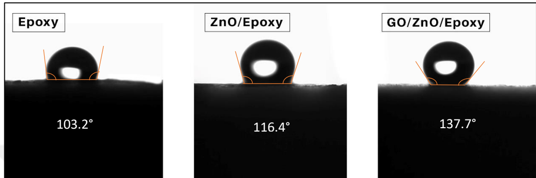
Figure 4.19. Contact angle of Epoxy coated substrate, ZnO/Epoxy coating and GO/ZnO/Epoxy coating.
