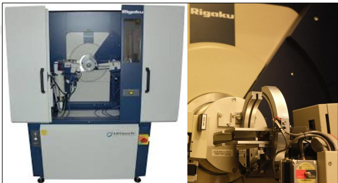
Figure 3.16. X-ray diffraction (XRD) instrument used for phase analysis.
