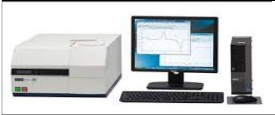
Figure 3.14. Automated system used in Thermogravimetric analysis.
